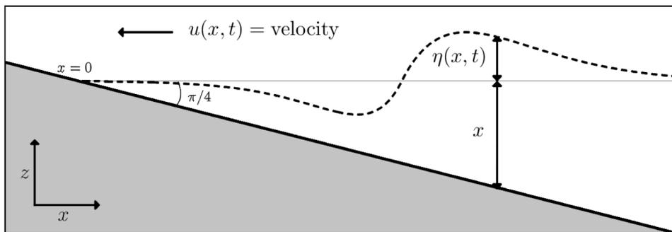
FIGURE 1. A sketch of the beach in the  $x$ - $z$  plane where  $\eta(x,t)$  is the water elevation over the unperturbed water level  $z = 0$  and  $H(x,t) = x + \eta(x,t)$  is the total perturbed water depth. The unperturbed shoreline occurs at  $x = 0$ ,  $z = 0$ .
