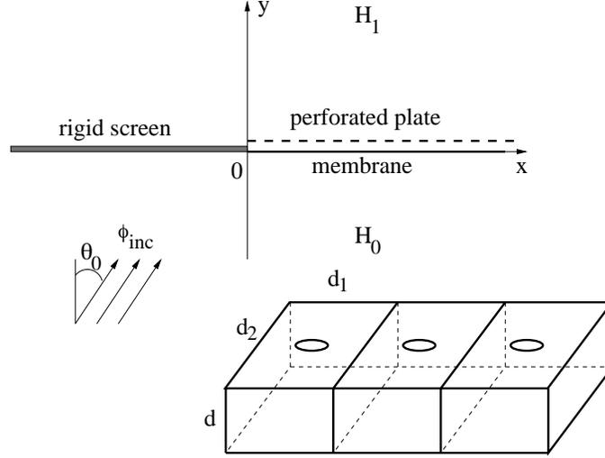
Figure 1: Sandwich panel attached to an acoustically rigid screen
