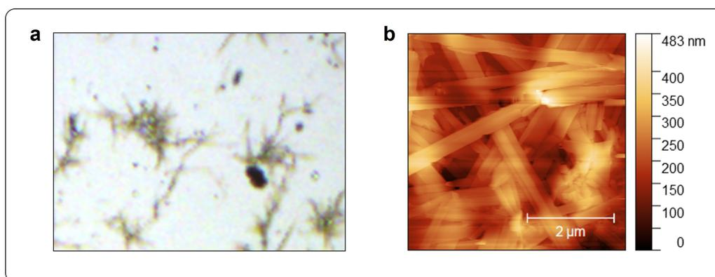
Figure 6: Optical and AFM image of clustered CBI-GCH crystals drop-casted on SiO<sub>2</sub>/Si wafer
