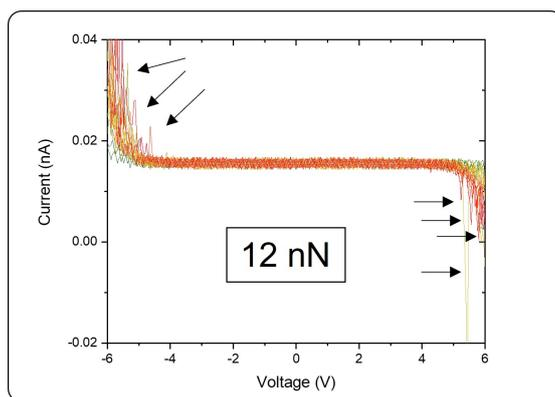
Figure 13: **IV spectroscopy** of a 35 nm thick CBI-GCH crystal. Black arrows highlight peaks. The tip force is set to 12 nN.
