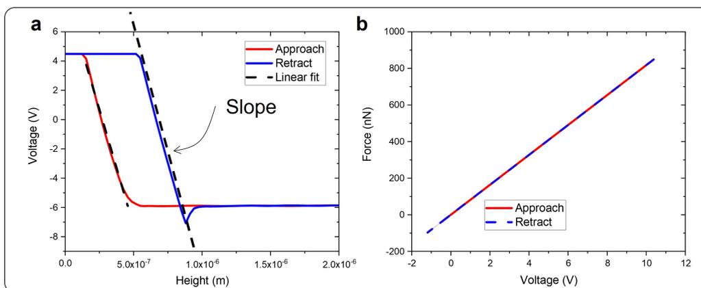
Figure 11: **F-z curve conversion of force.** (a) F-z curve with approach and retract curve. (b) Converted F-z force to derive the tip force in nN.
