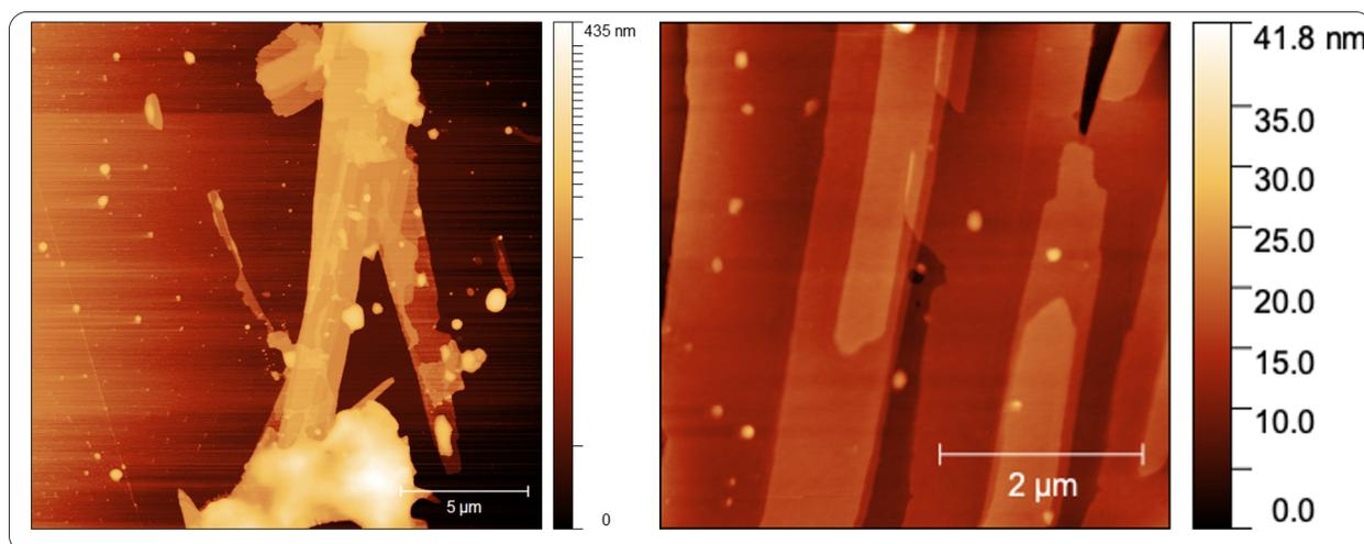
Figure 7: AFM topography of micrometer scale crystals deposited on SiO<sub>2</sub>/Si wafer
