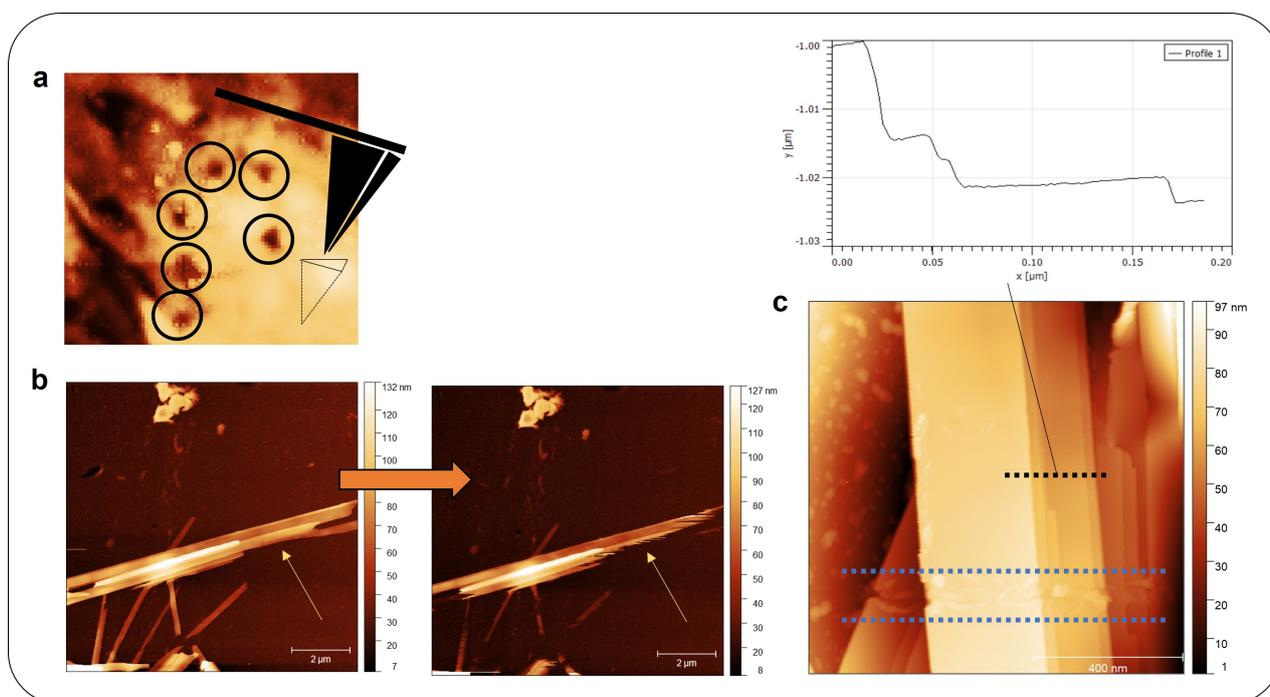
Figure 10: **AFM induced damage to CBI-GCH aggregates.** (a) Normal force induced tip indentation. (b) PeakForce induced damage to the crystal evident by sequential imaging of the same area. (c) CBI-GCH crystal showing local damage incurred by Amplitude Modulation Tapping Mode between the blue lines, by gently increasing the normal force. The black lines shows a cross-section line highlighting the stacked nature of the crystals.
