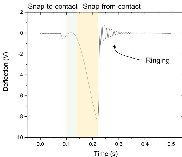
Figure 8: **PeakForce AFM force-distance spectroscopy**
