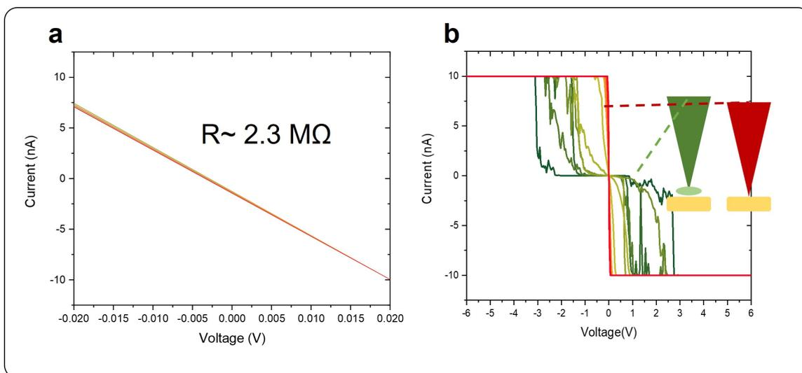
Figure 12: **IV spectroscopy of molecules coated tip on gold substrate.** (a) Ohmic contact resistance diamond tip on gold. (b) Observation of gradual change in IV behaviour (green) by sequential bias voltage ramping, until Ohmic resistance (red) is achieved. We conjecture tip contamination with molecular clusters.
