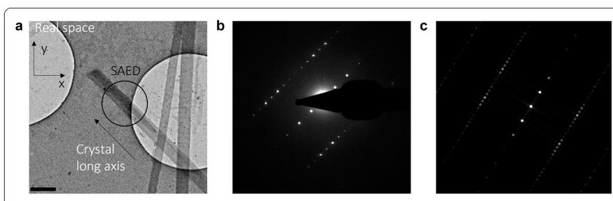
Figure 9: **TEM imaging** (a) Real space image of a crystal deposited on laceycarbon TEM grid. The black circle indicates selected area diffraction (SAED) location. (b) SAED showing high quality diffraction pattern. (c) Simulated FFT of a herringbone structure
