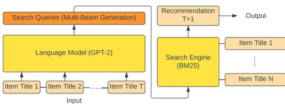
Figure 1: The architecture of the GPT4Rec framework.
