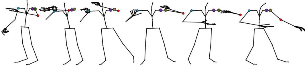
FIGURE 10. Illustration of the gesture performed in TVA_1 , where the operator grabs from a container a circuit board. The color annotations are based on the assumptions colored in (7). Colored joints indicate potential dependencies with other motion descriptors incorporated in the model: The orange indicates the transitioning assumption of RAy ; green reflects the intra-joint association with RAx and RAz ; blue highlights the inter-limb synergies with LAy ; purple is the serial intra-limb mediations with RSH2y and red the non-serial intra-limb mediations with RFAy . The picture of the recording can also be visualized in Fig. 1a.
