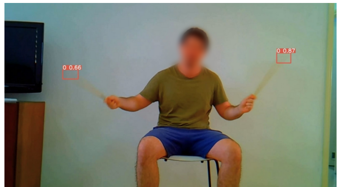
Fig. 4. Real-time tip detection under challenging conditions. The face is blurred for privacy purposes.
