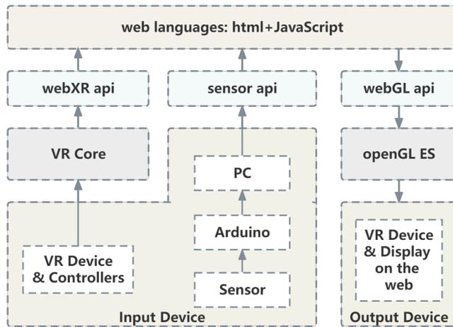
**Figure 4: Technical architecture.** This figure describes how the input signal is compiled into web language and then displayed in the web page of VR device. We convert VR and sensor applications into web language through webXR api and sensor api and then present 3D scenes on the web through WebGL api to let users experience the web in VR devices.
