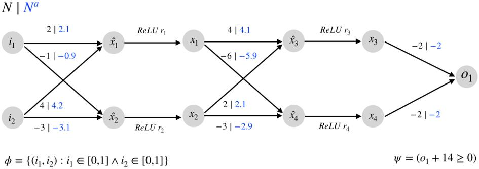
Fig. 2. Example original network  $N$  and its perturbation  $N^a$  (blue weights). Each layer consists of a linear function followed by the ReLU activation function.  $\phi$  is the input specification and  $\psi$  is the output specification.
