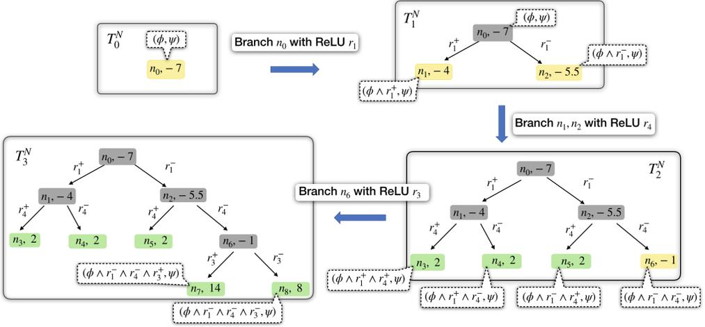
Fig. 3. Steps in Branch and Bound algorithm for complete verification of  $N$ . The nodes are labeled with a name and the  $LB_N(n)$ . The nodes in the specification tree are annotated with their specifications. The edges are labeled with the branching predicates. Each step in BaB partitions unsolved specifications in  $T_i^N$  into specification splits in  $T_{i+1}^N$ . The proof is complete when all specification splits corresponding to the leaf nodes are solved.
