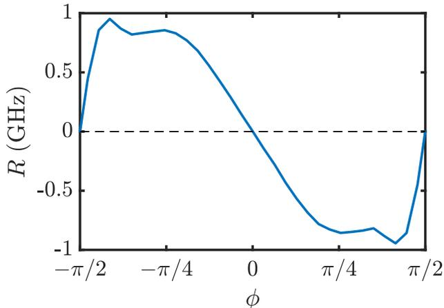
FIG. 4: The rotation rate,  $R$ , as a function of dihedral angle between phenyl rings  $\phi$ . Each  $R$  point is calculated via averaging over a trajectory with a length of  $\approx 1.6 \times 10^6$  ns. Voltage  $\mathcal{V} = 5V$ .
