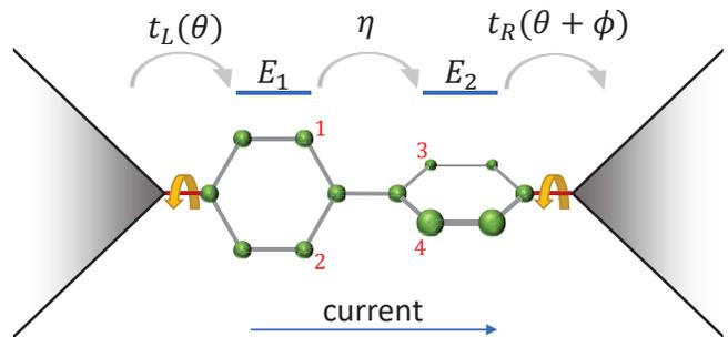
FIG. 1: Schematic of the model system. A biphenyl based molecule (green) connects two graphene electrodes. The molecule represents a rigid rotator. The dihedral angle between the two phenyl rings, which is critical for motor functionality, can be adjusted by the inclusion of appropriate side groups to atoms 1,2,3, and 4. An applied current induces a directional rotation about the red bonds when the dihedral angle between the phenyl rings is non-zero.
