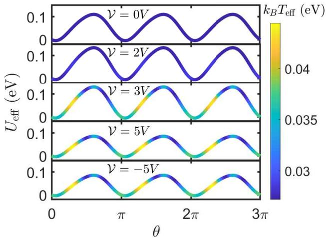
FIG. 2:  $U$  calculated according to (12) with  $k_B T_{\text{eff}}$  overlaid on top for different voltages. The nonhomogeneous temperature with local hot spots is the manifestation of the Landauer blowtorch effect. Dihedral angle between phenyl rings:  $\phi = -\pi/4$ .
