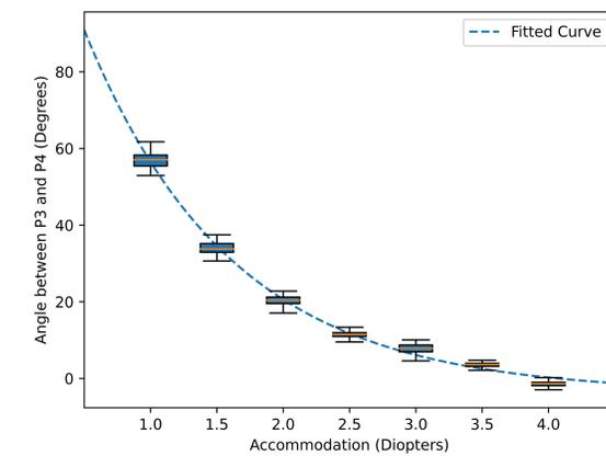
Figure 6: Accommodation versus angle between P3&P4 measured with one subject. Error bars indicate extremities and quartile range using 300 frames collected in 6 seconds after allowing for 2-3 seconds for transition.
