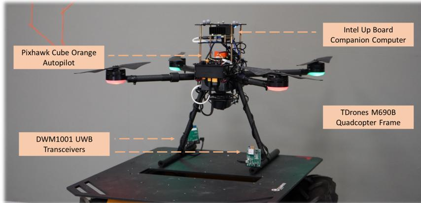
Fig. 4: Illustration of the UAV and UWB sensors used in our experiments.
