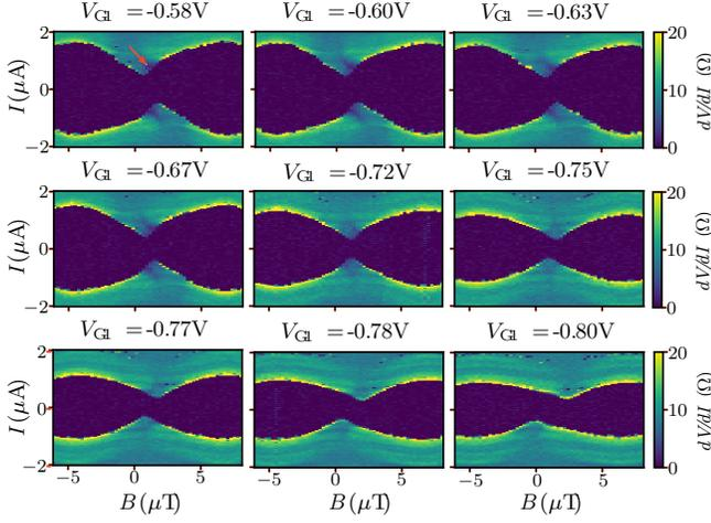
Figure 7. SQUID oscillation at different gate voltage configurations.  $V_{G2}$  is fixed at  $-0.5$  V, while  $V_{G1}$  is swept from  $-0.57$  V to  $-0.8$  V. The asymmetry in the SQUID oscillations follows the asymmetry in critical current between the two junctions. We have  $I_{c1}(V_{G1} = -0.57$  V)  $>$   $I_{c2}(V_{G2} = -0.5$  V) and  $I_{c1}(V_{G1} = -0.8$  V)  $<$   $I_{c2}(V_{G2} = -0.5$  V).
