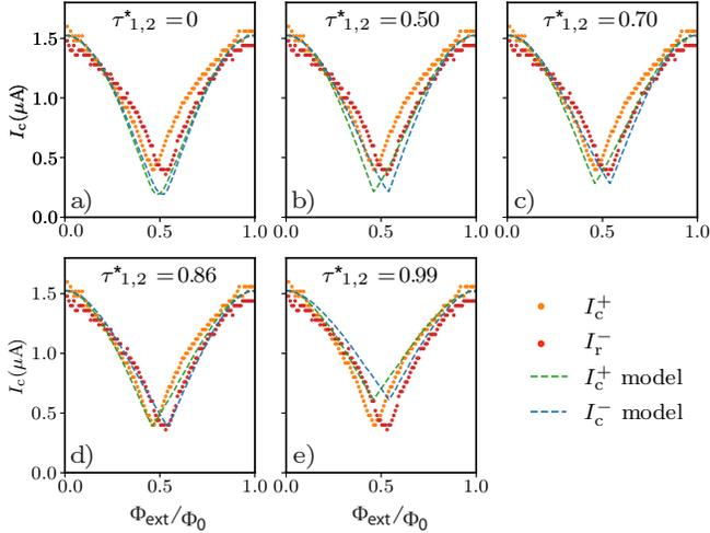
Figure 8. Sequence of simulations for  $I_c^+$  (green dashed curves) and  $I_c^-$  (blue dashed curves) to measured (upsweep) data  $I_c^+$  (orange dots) and  $I_c^-$  (red dots). In (a) a sinusoidal CPR with the estimated loop inductance asymmetry is considered, while in graphs (b)-(e) the effective transparencies  $\tau^*$  of the junctions are increased. Further details are given in the text.
