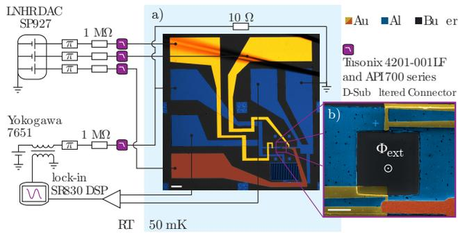
Figure 4. (a) False color optical image of the full device together with a sketch of the measurement setup. The scale bar is  $100 \mu\text{m}$ . (b) Zoom-in over the SQUID showing the loop area threaded by the external flux  $\Phi_{\text{ext}}$ . The electron density in the junction region is tuned via a set of gates coloured in yellow and brown. The scale bar is  $3 \mu\text{m}$
