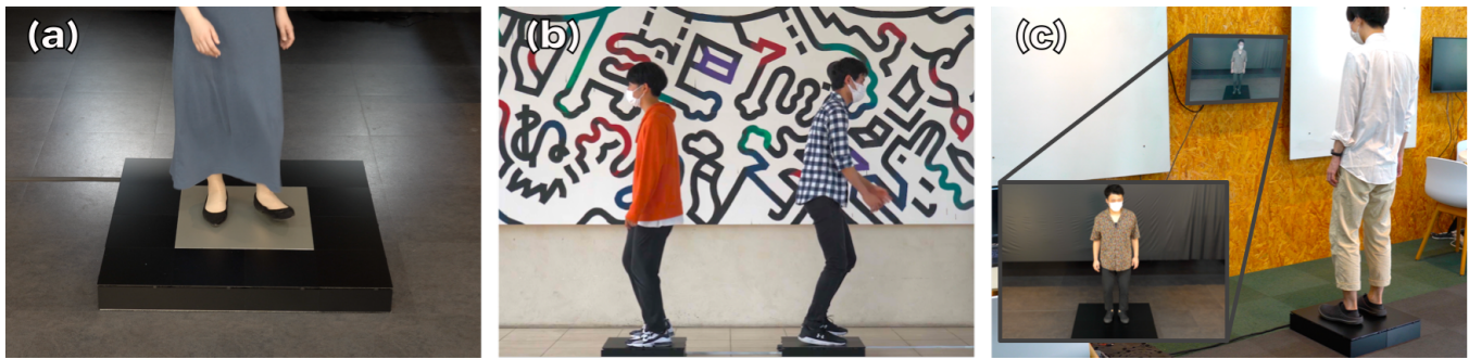
Figure 1: (a) SolefulTap provides tapping sounds and haptic stimulus from a floor-type impact display in response to the user's step motion. (b) Two users can tap dance in unison without directly seeing each other by using the sensation of their soles. (c) By recording the performance data, users can learn tap dancing steps multimodally through visual, audio, and haptic stimuli.
