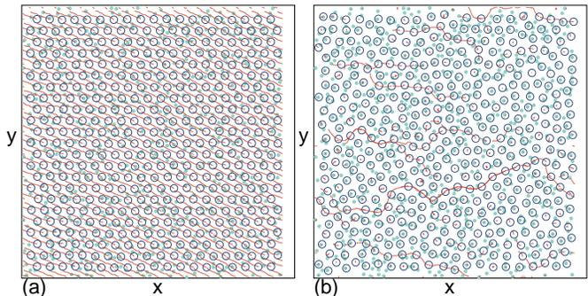
FIG. 4: The pinning site locations (filled circles), skyrmion locations (open circles), and trajectories (lines) for the system in Fig. 3 with  $T = 0$ . (a) At  $A_s = 3.0$  just above depinning, the flow is elastic. (b) At  $A_s = 0.5$ , the skyrmions are disordered and the depinning is plastic.
