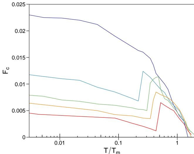
FIG. 12: The critical depinning force  $F_c$  vs  $T/T_m$  for the system in Fig. 9 at varied skyrmion density  $n_s = 0.2, 0.3, 0.4, 0.5,$  and  $0.6$ , from top to bottom. For  $n_s = 0.2$ , the system is disordered even at  $T/T_m = 0$  and there is no peak effect.
