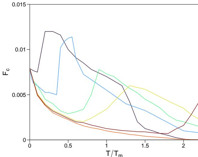
FIG. 14:  $F_c$  vs  $T/T_m$  for the same system from Fig. 9 with  $n_s = 0.4$  at  $\kappa = 3, 2, 1, 0.75, 0.5,$  and  $0$  from top to bottom. The peak effect shifts to higher temperatures as  $\kappa$  decreases. Here the curves have been normalized to  $T_m$  for the  $\kappa = 2.0$  system.
