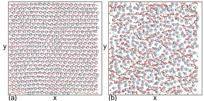
FIG. 11: The pinning site locations (filled circles), skyrmion locations (open circles), and trajectories (lines) for the system in Fig. 8 at  $F_D = 0.02$ . (a)  $T/T_m = 0.28$  where the flow is elastic. (b)  $T/T_m = 1.74$  where the flow is fluid.
