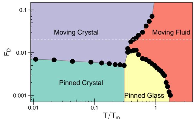
FIG. 8: Dynamic phase diagram as a function of  $F_D$  vs  $T/T_m$  constructed from the velocity-force curves and  $P_6$  data in Figs. 6 and 8 showing a pinned crystal, moving crystal, pinned glass, and moving glass. The horizontal dashed line indicates the value of  $F_D$  at which the velocity and skyrmion Hall angle data in Fig. 9 were obtained.
