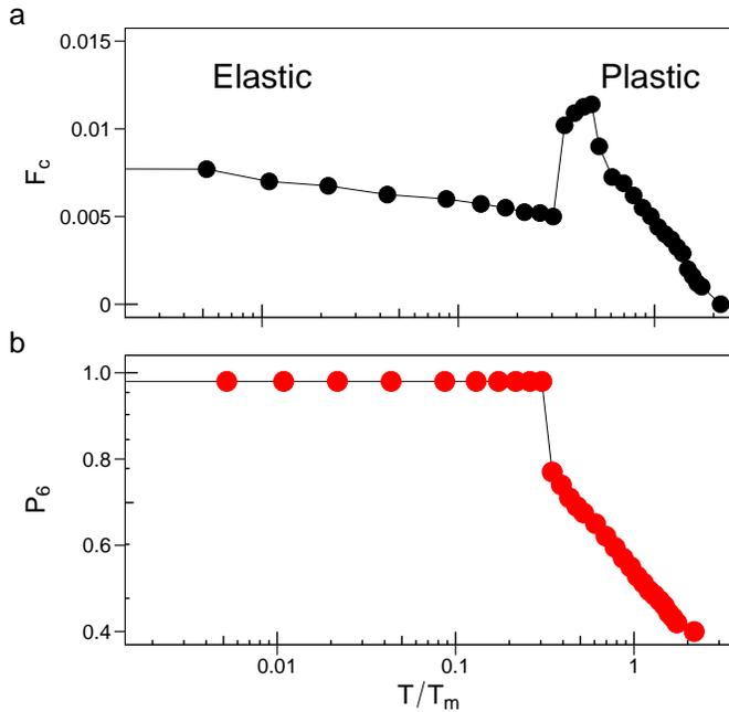
FIG. 6: (a)  $F_c$  vs  $T/T_m$  obtained from the velocity-force curves for the system in Fig. 5. (b) The corresponding  $P_6$  vs  $T/T_m$ , showing that the increase in  $F_c$  is associated with a disordering transition. NOTE THAT CHARLES SENT EXTRA IMAGES TO USE AS INSETS
