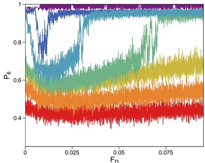
FIG. 7:  $P_6$  vs  $F_D$  for the system in Fig. 5 for  $T/T_m = 0.174, 0.348, 0.608, 0.869, 1.087, 1.304,$  and  $1.74$ , from top to bottom. For  $T/T_m < 1.0$ , the system dynamically orders into a moving crystal at higher drives.
