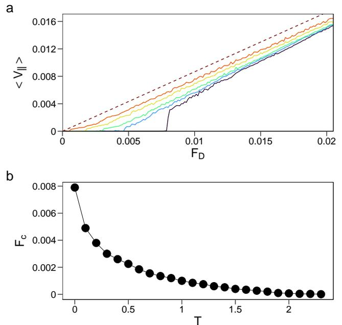
FIG. 1: (a) The skyrmion velocity  $\langle V_{\parallel} \rangle$  in the direction of the applied drive vs  $F_D$  in a system with fixed skyrmion-skyrmion interaction strength  $A_s = A_s^0$  at temperatures  $T = 0, 0.1, 0.2, 0.6,$  and  $1.4$ , from bottom to top. The dashed line is the expected response in the absence of pinning. (b) The critical depinning force  $F_c$  vs  $T$  for the system in (a). The depinning threshold decreases monotonically with increasing  $T$ .
