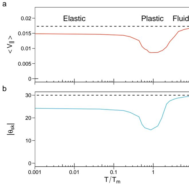
FIG. 9: (a)  $\langle V_{||} \rangle$  vs  $T/T_m$  for a slice at  $F_D = 0.02$ , above the depinning force, from the phase diagram in Fig. 8. There is a dip across the order to disorder transition. (b) The corresponding skyrmion Hall angle  $|\theta_{sk}|$  vs  $T/T_m$ , which also shows a dip. For  $T/T_m > 1.0$ , the values of both quantities approach the  $F_p = 0$  values (dashed lines).
