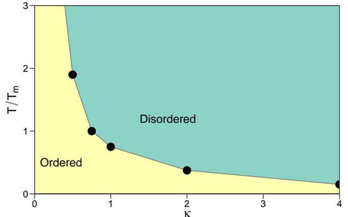
FIG. 15: Dynamic phase diagram of the order to disorder transition as a function of  $T$  vs  $\kappa$  for the system in Fig. 13 with  $n_s = 0.4$ . Here the temperature has been normalized using  $T_m$  for the  $\kappa = 2.0$  system.
