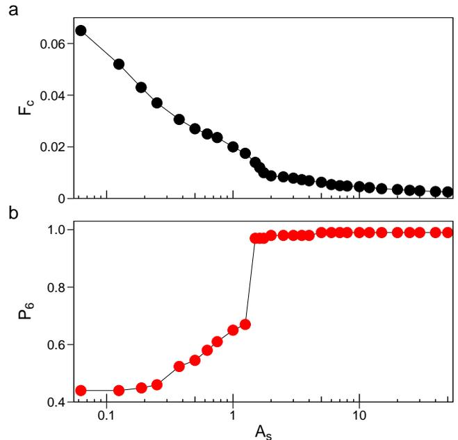
FIG. 3: (a)  $F_c$  vs  $A_s$  for the system in Fig. 2 with  $T = 0$ . (b) The corresponding fraction  $P_6$  of sixfold-coordinated skyrmions vs  $A_s$ . As  $A_s$  decreases,  $F_c$  increases, with a more rapid increase appearing at the order to disorder transition near  $A_s = 1.25$ .
