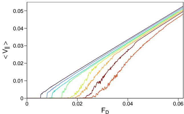
FIG. 2:  $\langle V_{||} \rangle$  vs  $F_D$  for the system in Fig. 1 at  $T = 0$  for modified skyrmion-skyrmion interaction strengths of  $A_s = 6.0, 3.0, 1.75, 1.5, 1.25, 1.0, 0.75$  and  $0.5$ , from top to bottom. The depinning threshold monotonically increases with decreasing  $A_s$ . The depinning transition is elastic for  $A_s > 1.25$  and plastic for  $A_s \leq 1.25$ .
