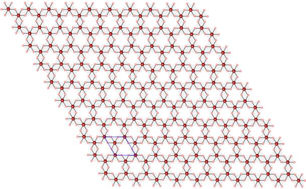
FIG. 4. CrI<sub>3</sub> structure. The atoms of chromium and iodine are represented by red and pink spheres, respectively. The unit cell of CrI<sub>3</sub> consists of two Cr atoms and six I atoms, with the Cr atoms forming a honeycomb structure.
