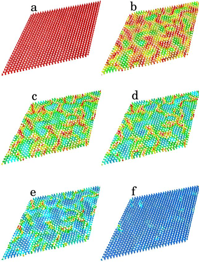
FIG. 5. Evolution of the magnetic structure of the system for the pulse fluence  $F_1 = 166 \text{ mJ/cm}^2$ . The fluence magnitude is sufficient to induce the magnetization reversal. The snapshots (a)-(f) correspond to 1.6 ps, 1.8 ps, 1.84 ps, 1.86 ps, 1.9 ps, and 2.04 ps, respectively. The color codes the orientation of the magnetic moments of the Cr atoms.
