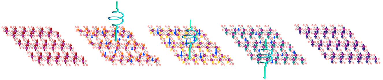
FIG. 1. Schematic representation of the optical magnetization switching in  $\text{CrI}_3$  monolayer. Here we demonstrate the system evolution in time (left to right). The monolayer is irradiated by circularly polarized light. Optical pumping leads to the formation of excitons carrying magnetic moment defined by the pump helicity which interact with the lattice magnetization of the sample.
