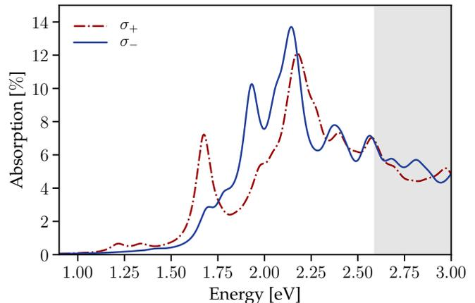
FIG. 3. Absorption spectrum of  $\text{CrI}_3$  sample for two circular polarizations. The solid line and the dashed line correspond to the  $\sigma_-$  and  $\sigma_+$  polarizations, respectively. The bandgap energy  $E=2.59 \text{ eV}$  is indicated by gray shading.
