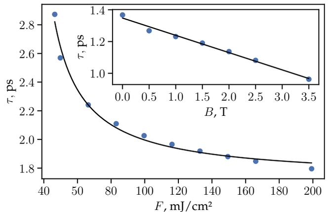
FIG. 8. Magnetization switching time  $\tau$  as a function of pump fluence  $F$ . Magnetization switching is achieved if the fluence of the pulse exceeds a critical value  $F_c \approx 46 \text{ mJ/cm}^2$ , at which the switching time diverges. The inset shows the switching time as a function of the lateral external magnetic field for the fluence of  $133 \text{ mJ/cm}^2$ .
