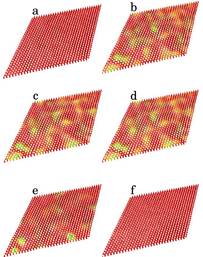
FIG. 6. Evolution of the magnetic structure of the system for the pulse fluence  $F_2 = 33 \text{ mJ/cm}^2$ . The fluence magnitude is insufficient to induce the magnetization reversal. The snapshots (a)-(f) correspond to 2.2 ps, 2.76 ps, 2.98 ps, 3.2 ps, 4.4 ps, and 8.0 ps, respectively. The color codes the orientation of the magnetic moments of the Cr atoms. This case corresponds to the dashed line in Fig. 7.
