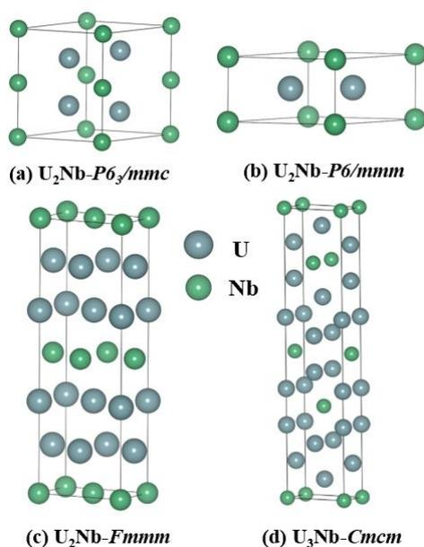
**Fig. 2** (color online) Crystal structures of  $U_2Nb$  in the phase of (a)  $P6_3/mmc$  (being stable up to approximately 21.6 GPa), (b)  $P6/mmm$  (stable within approximately 21.6–368 GPa) and (c)  $Fmmm$  (beyond 368 GPa). (d) The predicted  $Cmcm$  structure of  $U_3Nb$ .
