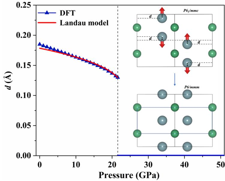
**Fig. 14** (color online) Evolution of the order parameter  $d$  from structure  $P6_3/mmc$ - $U_2Nb$  to  $P6/mmm$ - $U_2Nb$  as a function of pressure. The discontinuous jump at the transition pressure is evident. Inset schematics illustrate the atomic rearrangement during the structural transition, in which bold-line box represents the primitive cell of  $P6/mmm$ - $U_2Nb$ .
