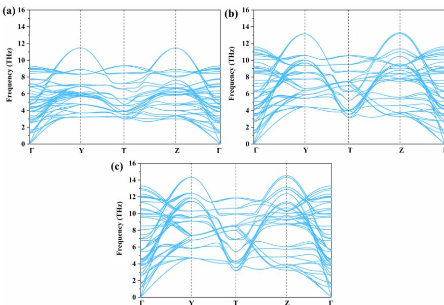
**Fig. S6.** Calculated phonon spectra of  $Cmcm$ - $U_3Nb$  at (a) 100 GPa, (b) 200 GPa and (c) 300 GPa.
