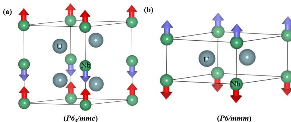
**Fig. S7.** The vibrational modes of the optical branches with the highest frequency at the gamma point for the (a)  $P6_3/mmc$  and (b)  $P6/mmm$  phases of  $U_2Nb$ .
