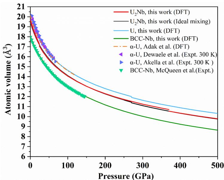
**Fig. S10.** Calculated equation of state of  $U_2Nb$ ,  $\alpha$ -U (0–270 GPa),  $\gamma'$ -U (270–500 GPa), and BCC-Nb at zero Kelvin as compared to previous DFT and experimental data [5–8]. The hypothetical U-Nb solid solution with a composition of U:Nb=2:1 as estimated by the ideal mixing model is also shown for comparison.
