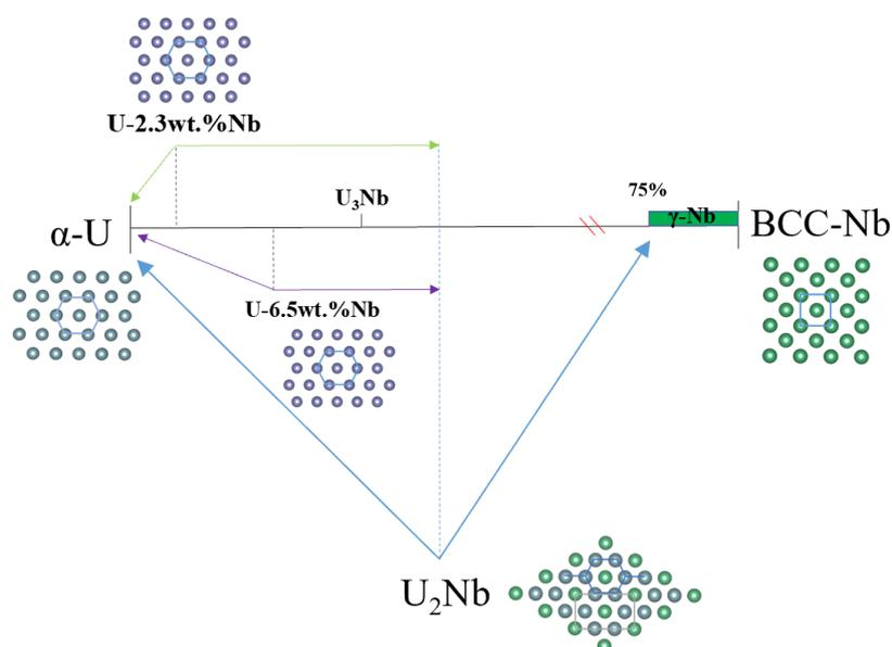
**Fig. 16** (color online) Schematic decomposition route of aged metastable  $\alpha'$  (U-2.3 wt. % Nb) or  $\alpha''$  (U-6.5 wt. % Nb) phase in U-Nb system via the intermediate  $U_2Nb$  ordered phase.
