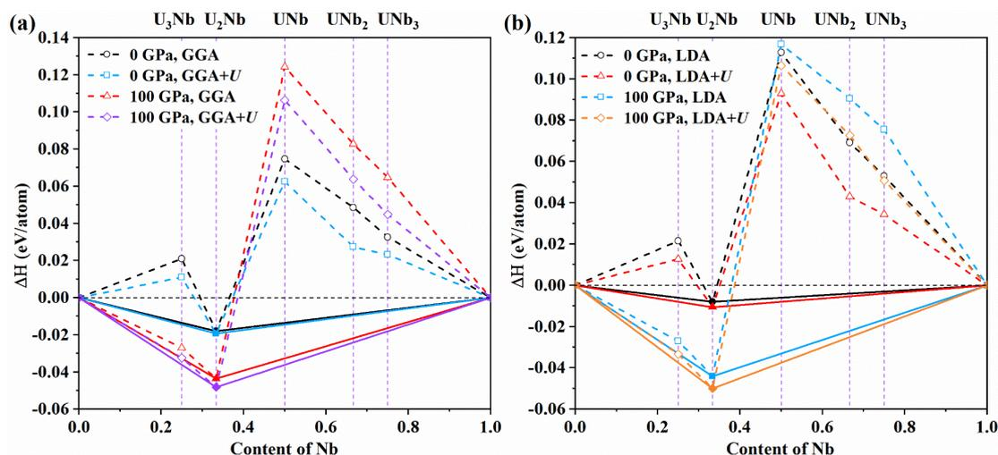
**Fig. 3** (color online) Convex hulls of predicted structures at 0 and 100 GPa using (a) GGA and GGA+ $U$  and (b) LDA and LDA+ $U$  ( $U=1.0$  eV). Solid lines connect thermodynamically stable phases at the given pressure, and dashed-line connections represent unstable or metastable phases.
