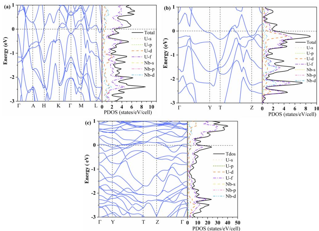
**Fig. S11.** Electronic band structures (left panel) and projected density of states (right panel) of (a)  $P6/mmm$ - $U_2Nb$  at 100 GPa, (b)  $Fmmm$ - $U_2Nb$  at 400 GPa and (c)  $Cmcm$ - $U_3Nb$  at 100 GPa.
