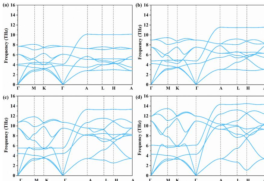
**Fig. S4.** Calculated phonon spectra of  $P6/mmm$ - $U_2Nb$  at (a) 50 GPa, (b) 100 GPa, (c) 200 GPa and (d) 300 GPa.
