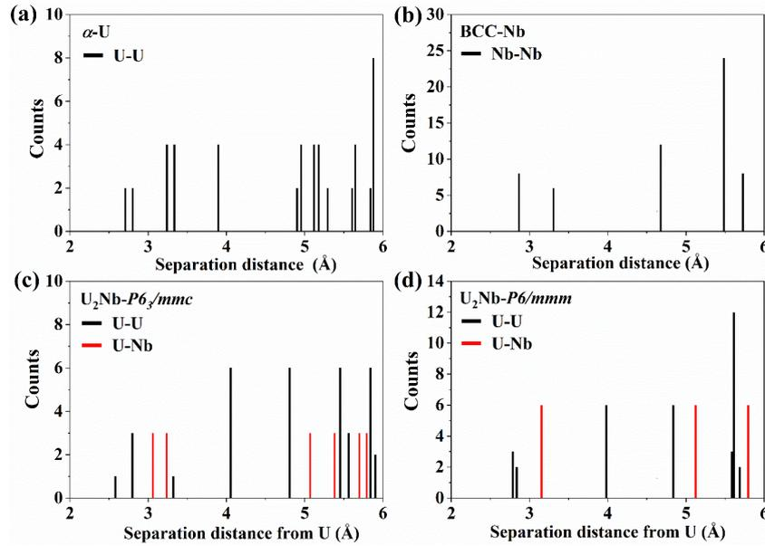
**Fig. 6** (color online) Histograms of interatomic separations for (a)  $\alpha$ -U, (b) BCC-Nb, (c)  $P6_3/mmc$ - $U_2Nb$ , and (d)  $P6/mmm$ - $U_2Nb$  at zero pressure.
