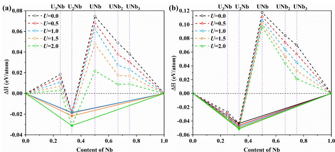
**Fig. 4** (color online) Convex hulls of different  $U$  values calculated by GGA+ $U$  ( $U=0, 0.5, 1.0, 1.5, 2.0$  eV).
