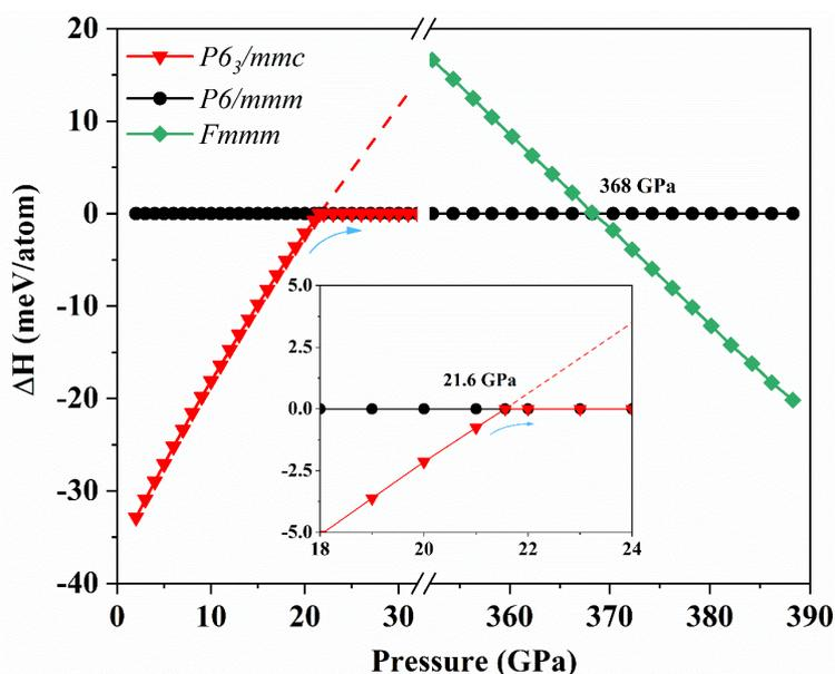
**Fig. 9** (color online) Enthalpy difference of  $U_2Nb$  in  $P6_3/mmc$  and  $Fmmm$  phases with respect to the  $P6/mmm$  phase. The dashed-line indicates the region where  $P6_3/mmc$  becomes spontaneously unstable.
