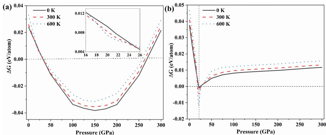
**Fig. S15.** Calculated formation Gibbs free energy  $\Delta G$  as a function of pressure at different temperatures of 0, 300 and 600 K for  $Cm\bar{c}m$ - $U_3Nb$ . The vertical dotted-line in (b) corresponds to a pressure of 21.6 GPa. The reference terminal states are  $\alpha$ -U and BCC-Nb for (a), and  $\alpha$ -U and  $U_2Nb$  for (b).
