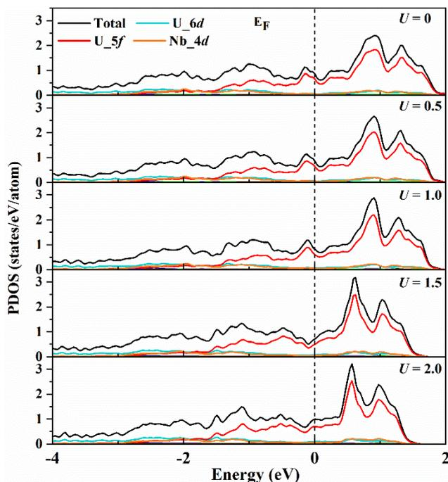
**Fig. S20.** Calculated projected density of states (PDOS) with different  $U$  values for  $P6_3/mmc$ - $U_2Nb$  at 0 GPa.
