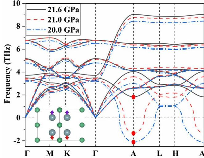
**Fig. 11** (color online) Calculated phonon spectra of  $P6/mmm$ - $U_2Nb$  at 20.0, 21.0 and 21.6 GPa. The vibrational soft mode at high symmetry point  $A$  ( $0, 0, 1/2$ ) is marked by the solid circles and shown in the inset.
