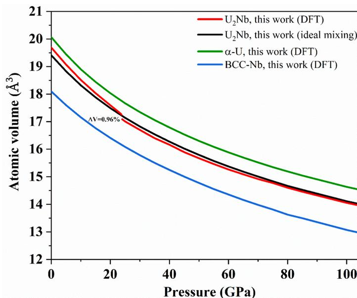
**Fig. 8** (color online) Calculated equation of state of  $U_2Nb$ ,  $\alpha$ -U, and BCC-Nb at 0 K. The hypothetical U-Nb solid solution with a composition of U:Nb=2:1 as estimated by using the ideal mixing model is also shown for comparison.
