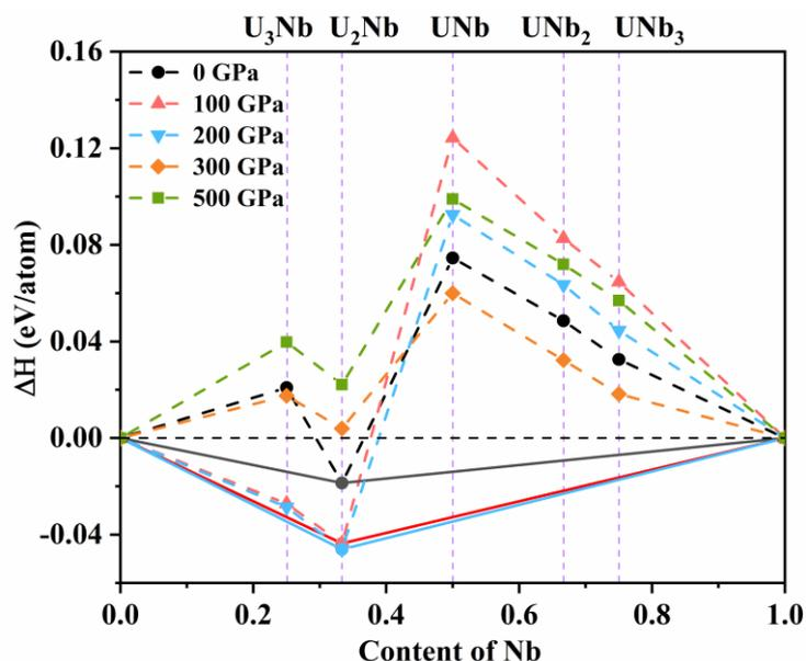
**Fig. 1** (color online) Convex hulls of predicted structures at different pressures. Solid lines connect thermodynamically stable phases at the given pressure, and dashed-line connections represent unstable or metastable phases.
