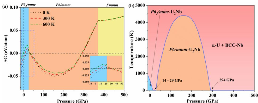
**Fig. 15** (color online) (a) Calculated formation Gibbs free energy ( $\Delta G$ ) of  $U_2Nb$  from -10 to 500 GPa with respect to  $\alpha$ -U and BCC-Nb at 0, 300 and 600 K. The respective
