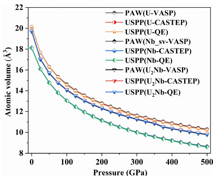
**Fig. S17.** Calculated equation of state of  $U_2Nb$ , U and Nb at zero Kelvin with different pseudopotentials.
