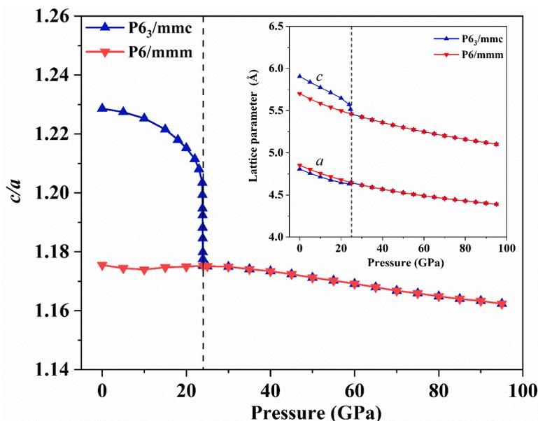
**Fig. 10** (color online) Variation of lattice vectors  $a$  and  $c$ , and their ratio  $c/a$  with pressure in  $P6_3/mmc$ - $U_2Nb$  and  $P6/mmm$ - $U_2Nb$  phases, respectively. The dashed-vertical line indicates the transition pressure.
