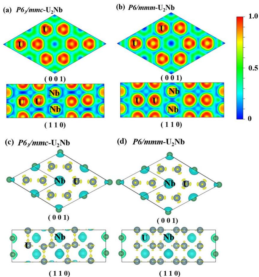
**Fig. S13.** Electron localization function (ELF) of (a)  $P6_3/mmc-U_2Nb$  and (b)  $P6/mmm-U_2Nb$  at 21.6 GPa. The differential charge density (isosurface =  $0.02 e/\text{bohr}^3$ ) of (c)  $P6_3/mmc-U_2Nb$  and (d)  $P6/mmm-U_2Nb$  at 21.6 GPa. The blue color indicates the loss of electrons and yellow color represents the gain of charge.
