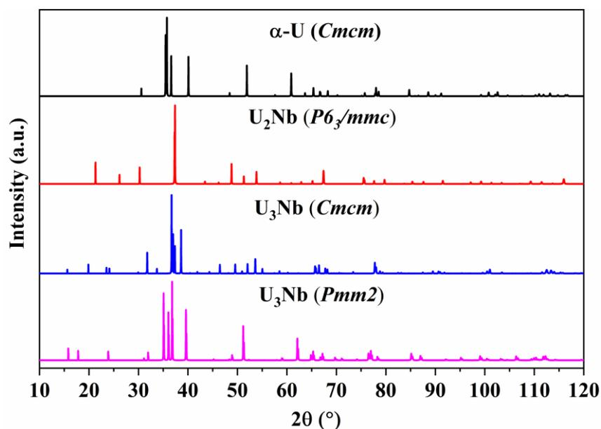
**Fig. S8.** Simulated X-ray diffraction pattern for  $\alpha$ -U,  $P6_3/mmc$ - $U_2Nb$ ,  $Cmcm$ - $U_3Nb$ , and  $Pmm2$ - $U_3Nb$  by using a wave-length of  $\lambda = 1.54 \text{ \AA}$  at 0 GPa.
