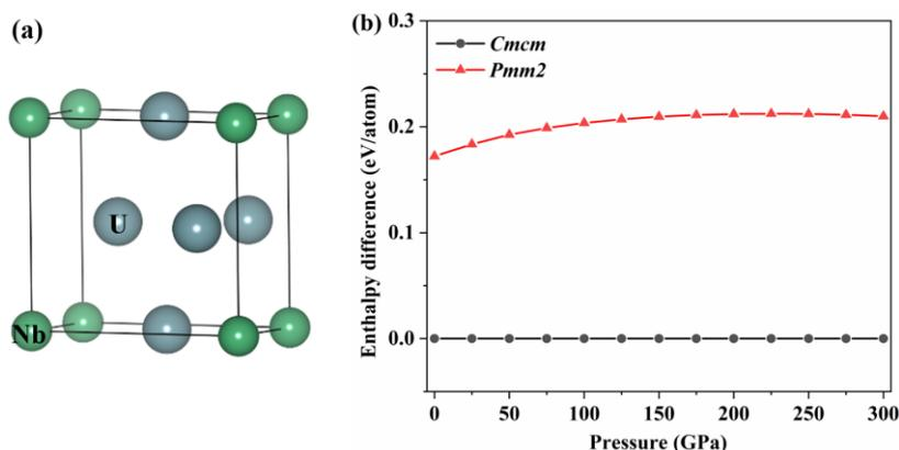
**Fig. S2.** (a) The structure of  $U_3Nb$  ( $Pmm2$ , which is a distorted  $Cu_3Au$ -type ( $L1_2$ ) structure) relaxed from the candidate structure proposed by Zhang et al. [4] which is unstable. (b) Calculated enthalpy difference between  $Pmm2$ - $U_3Nb$  and our newly predicted  $Cmc$ - $U_3Nb$  as a function of pressure.
