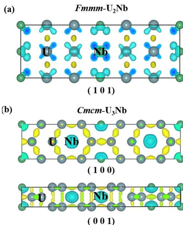
**Fig. S14.** Differential charge density (isosurface =  $0.02 e/\text{bohr}^3$ ) of (a) *Fmmm-U<sub>2</sub>Nb* at 400 GPa and (b) *Cmc-U<sub>3</sub>Nb* at 200 GPa. The blue color indicates the loss of electrons and yellow color represents the gain of charge between U atoms.
