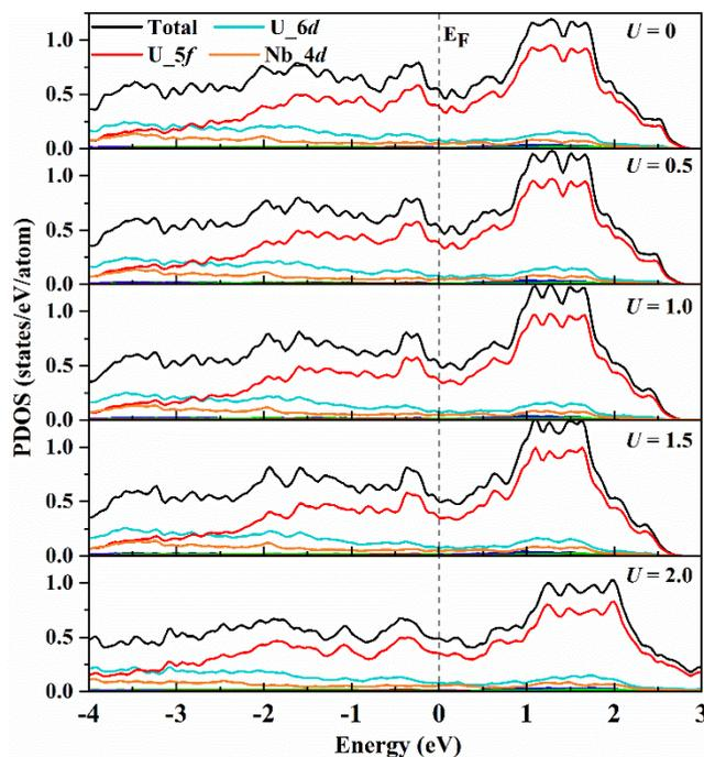
**Fig. S22.** Calculated projected density of states (PDOS) with different  $U$  values for *Cmcmm-U<sub>3</sub>Nb* at 100 GPa.
