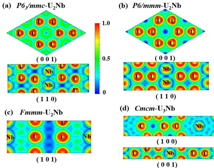
**Fig. S12.** Electron localization function (ELF) of (a)  $P6_3/mmc$ - $U_2Nb$  at 0 GPa, (b)  $P6/mmm$ - $U_2Nb$  at 200 GPa on the plane of (0 0 1) and (1 1 0), (c)  $Fmmm$ - $U_2Nb$  at 400 GPa on the plane of (1 0 1) and (d)  $Cmcm$ - $U_3Nb$  at 200 GPa on the plane of (1 0 0) and (0 0 1). ELF isosurfaces are drawn along with the value from 0 (blue) to 1.0 (red).
