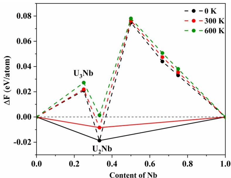
**Fig. S16.** Calculated formation free energy  $\Delta F$  at zero pressure at temperatures of 0, 300, and 600 K.
