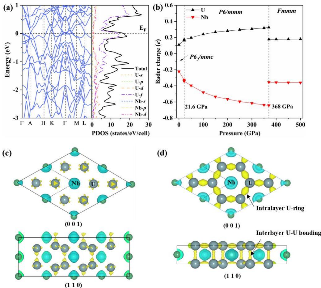
**Fig. 7** (color online) (a) Electronic band structure and projected DOS of  $P6_3/mmc$ - $U_2Nb$  at zero pressure. (b) The averaged Bader charge of U and Nb atoms in each  $U_2Nb$  phase. (c) Differential charge density (isosurface =  $0.02 e/\text{bohr}^3$ ) of  $P6_3/mmc$ - $U_2Nb$  at 0 GPa, and (d)  $P6/mmm$ - $U_2Nb$  at 200 GPa. The blue color indicates the loss of electrons from Nb atoms and the yellow color represents the grain of electrons between U atoms.
