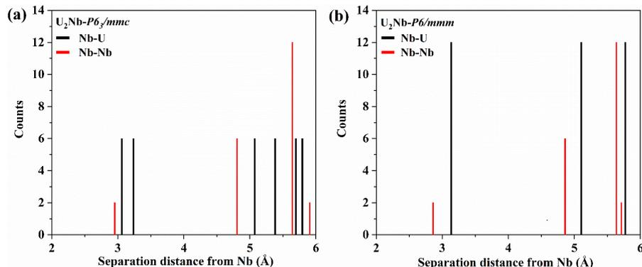
**Fig. S9.** Interatomic separation histograms for (a)  $P6_3/mmc$ - $U_2Nb$  and (b)  $P6/mmm$ - $U_2Nb$  at zero pressure.
