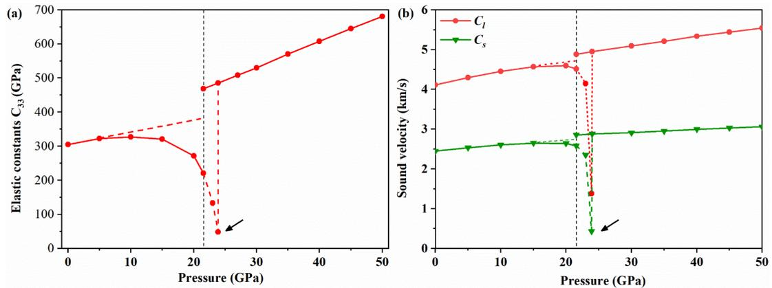
**Fig. 12** (color online) Variation of (a) elastic constant  $C_{33}$  and (b) shear ( $C_s$ ) and longitudinal ( $C_l$ ) sound velocity with pressure. The vertical dotted-line indicates the first-order transition pressure, whereas the arrows mark the underlying  $\lambda$  transition buried by the former and exhibits divergence in the elastic constant  $C_{33}$  and sound velocities.
