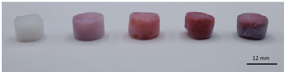
Figure S1. Aeroglass (AG) functionalized with increasing concentration (from left to right) of gold nanoparticles.
