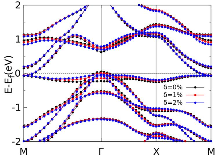
**Figure S6.** The band structure of strained single-layer Fe<sub>2</sub>Se<sub>2</sub>. Black, red, blue points correspond to unit cells uniformly stretched by 0%, 1%, 2%, respectively.
