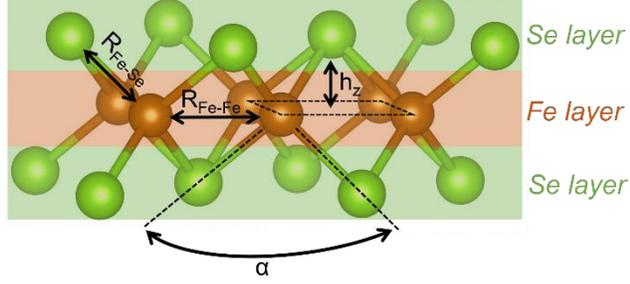
**Figure 5.** Schematic depicting the local lattice environments, involving the in-plane  $\text{FeSe}_4$  edge-sharing tetrahedral units, defined by the bond lengths ( $R_{\text{Fe-Se}}$  and  $R_{\text{Fe-Fe}}$ ), the anion height ( $h_z$ ) and Se-Fe-Se bond angle ( $\alpha$ ).
