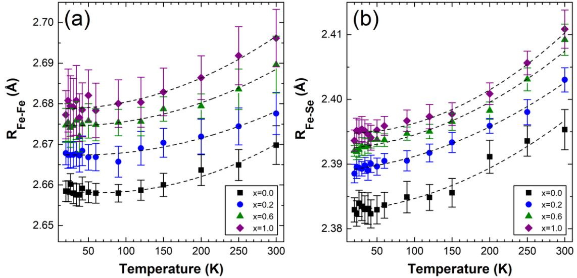
**Figure 6.** Temperature evolution of the bond correlations in the  $\text{Li}_x(\text{C}_5\text{H}_5\text{N})_y\text{Fe}_{2-z}\text{Se}_2$  ( $0 \leq x \leq 1$ ) series: (a) the Fe-Fe pairs of distances, extracted from the Fe K-edge, and (b) the Fe-Se pairs of bonds, extracted from the Se K-edge. The dashed lines are a guides to the eye.
