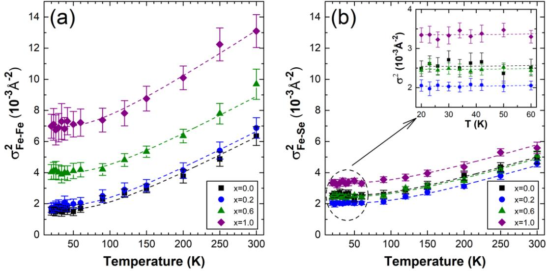
**Figure 7.** Temperature evolution of the MSRDs ( $\sigma^2$ ) for  $\text{Li}_x(\text{C}_5\text{H}_5\text{N})_y\text{Fe}_{2-z}\text{Se}_2$  ( $0 \leq x \leq 1$ ) samples: (a) for Fe-Fe pairs extracted from the Fe K-edge, and (b) for Fe-Se pairs extracted from the Se K-edge. Inset: Zoom in the temperature range (20-60) K revealing the subtle variations of the MSRDs. The dashed lines in (a, b) are the corresponding least square fits based on the correlated Einstein model (see text).
