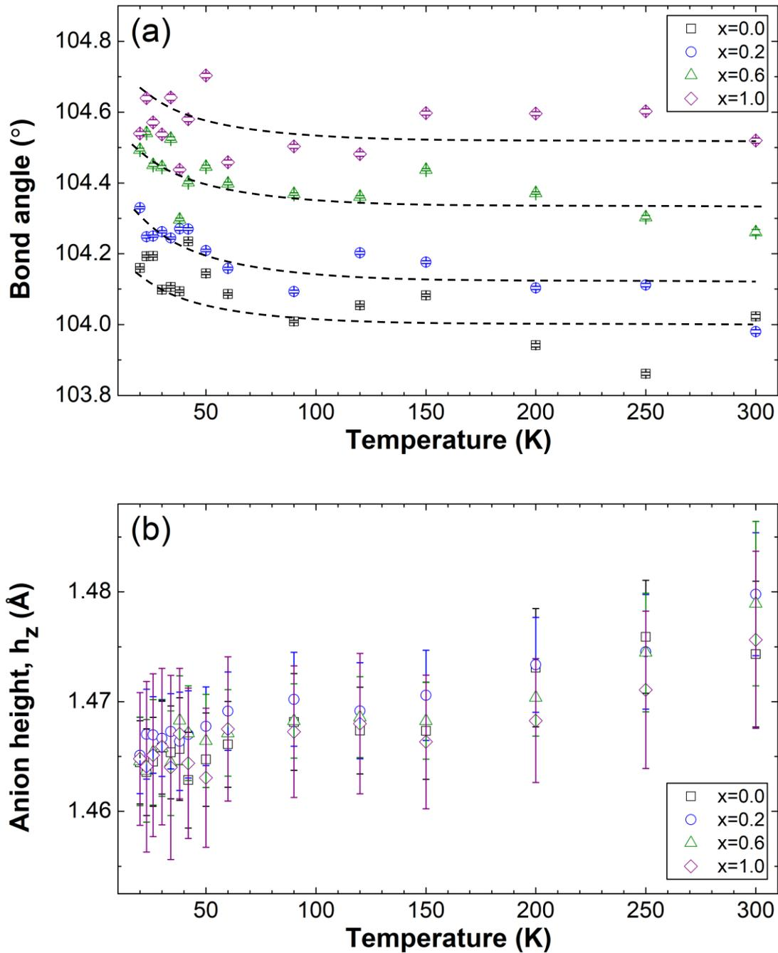
**Figure S4.** The temperature dependence of (a) the bond angle  $\alpha$  and (b) the anion height,  $h_z$ , determined from the intra-layer bond distances ( $R_{\text{Fe-Se}}$ ,  $R_{\text{Fe-Fe}}$ ) extracted from fitting the measured Fe K-edge EXAFS spectra of the  $\text{Li}_x(\text{C}_5\text{H}_5\text{N})_y\text{Fe}_{2-z}\text{Se}_2$  series. The dashed lines are a guide to the eye.
