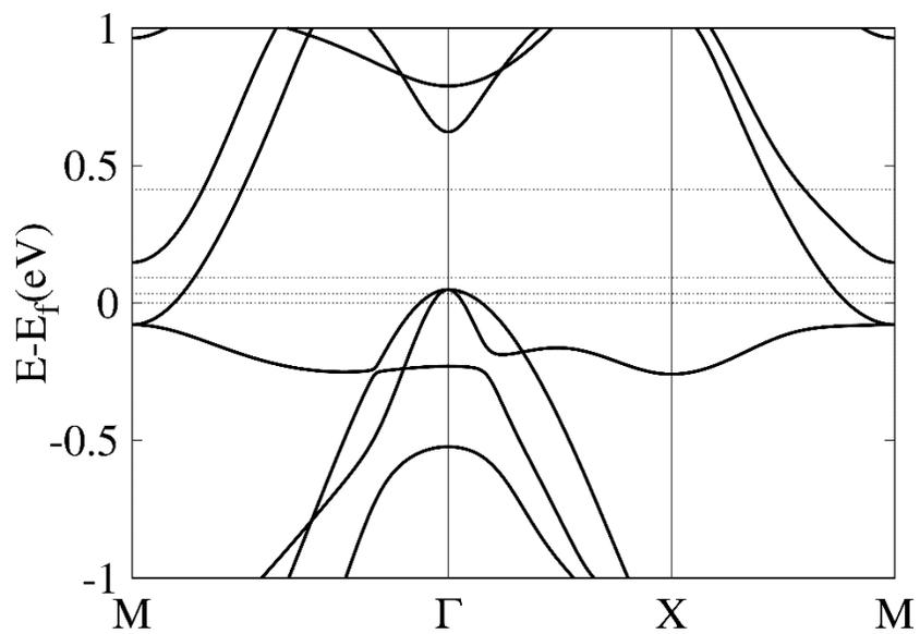
**Figure S7.** The band structure of the pristine single-layer  $\text{Fe}_2\text{Se}_2$ . The dashed lines represent the Fermi levels ( $E_f$ ) for different values of excess electrons per Fe atom, from bottom up at 0.0, 0.1, 0.2 and 0.5  $e/\text{Fe}$ .
