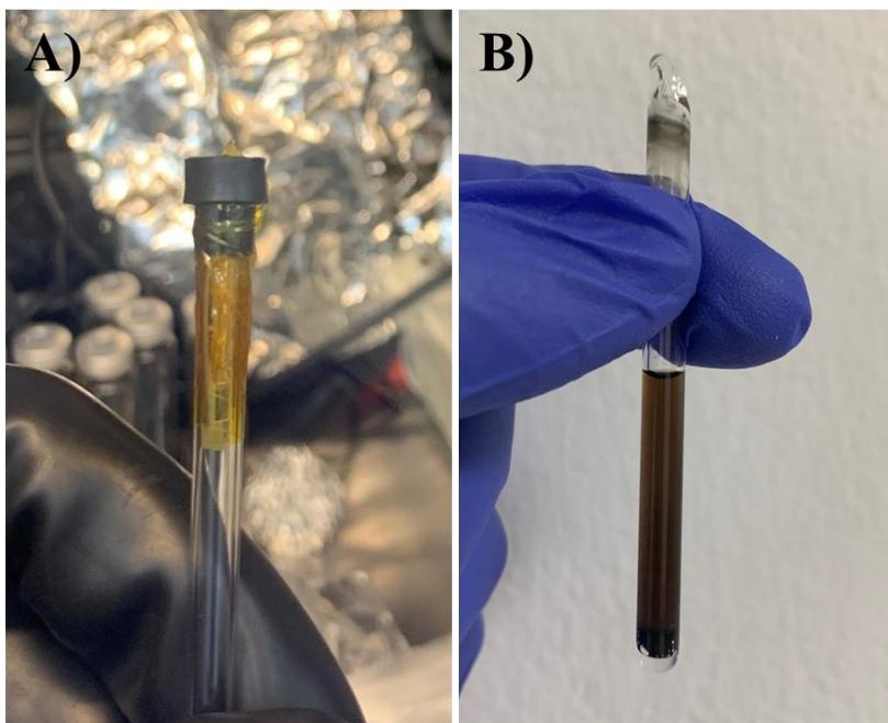
**Figure S2.** Photos of the quartz ampoules used for the AC magnetic susceptibility experiments. Example of ampule (A) covered with parafilm layer, closed with NMR plastic cap and sealed with Kapton tape, which showed no solvent evaporation after 7 days at 80°C; (B) flame-sealed ampoule, with “Li-PyH5-FeSe reactants in the mother liquid, used for magnetic measurement at variable times (i.e. 8 h, 18 h and 28 h).
