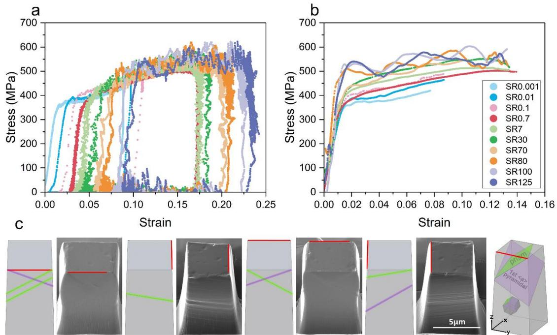
Figure 7 (a) The coupled engineering stress-strain curves for micropillar compression tests in P1 at both NSR and HSR. [Each test has shifted slightly along the X axis to aid visualisation.] (b) Smoothed stress-strain curves of the coupled P1 results; (c) SE micrographs and 3D models showing the relationship between pillars and slip planes for the four sides of the deformed pillar P1 at strain rate 125. [The red line annotation indicates the same pillar vertex for each micrograph.]
