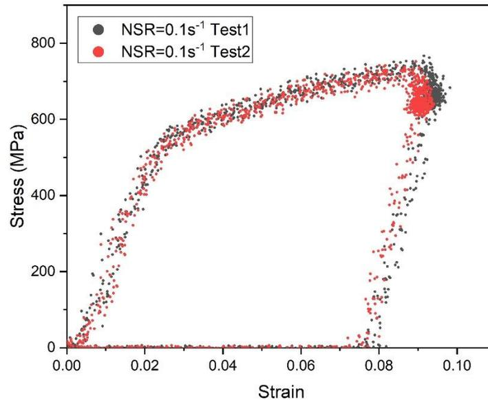
Figure 3 Two micropillar compression tests on the pillars in B1 with quasi-static strain rates  $0.1 \text{ s}^{-1}$ .
