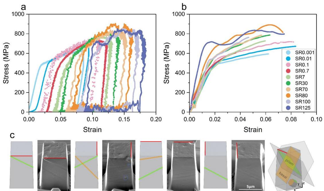
Figure 6 (a) The coupled engineering stress-strain curves for micropillar compression tests in B2 at both NSR and HSR. [Each test has shifted slightly along the X axis to aid visualisation.] (b) Smoothed stress-strain curves of the coupled B2 results; (c) SE micrographs and 3D models showing the relationship between pillars and slip planes for the four sides of the deformed pillar B2 at a strain rate of 100. [The red line annotation indicates the same pillar vertex for each micrograph.]
