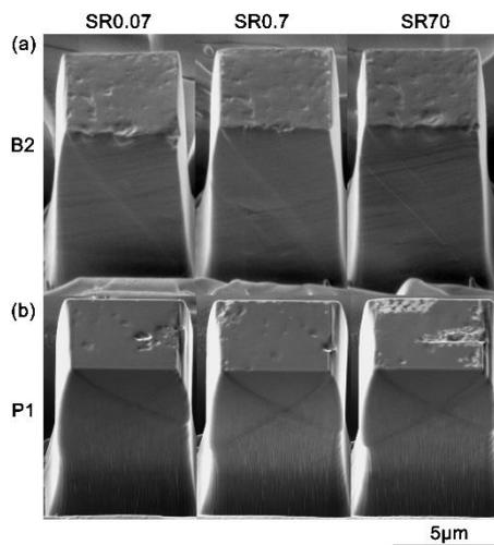
Figure 14 SE micrographs showing post-deformation micropillars in different grains B2 and P1, compressed with different strain rates. [The SE micrographs of other sides of the pillar can be found in Supplementary.]
