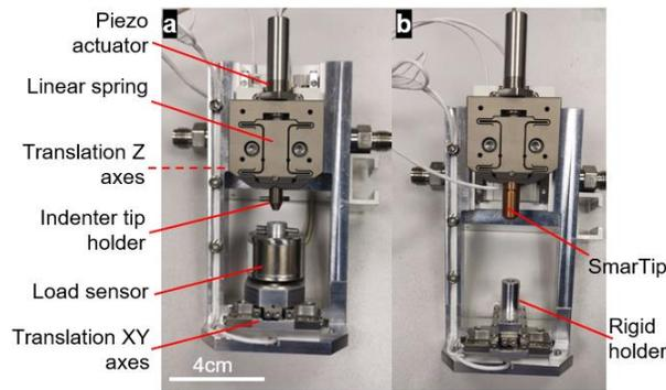
Figure 2 The hardware components of the Alemnis nanoindenter stages for different strain rate testing (a) quasi-static, and (b) high strain rate.
