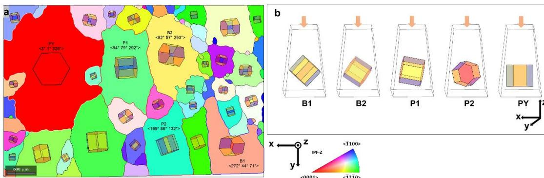
Figure 1 (a) An EBSD mapping with IPF-Z colouring and crystal shapes of the region of interest in the ‘blocky alpha’ large grain Zircaloy-4. (b) A schematic of the micropillar with the hcp crystal shape representing its orientation inside.
