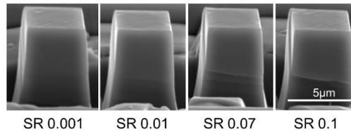
Figure 9 The SE images of deformed micropillar in P2 with different quasi-static strain rates. (The *in situ* videos can be found in the supplementary figures.)
