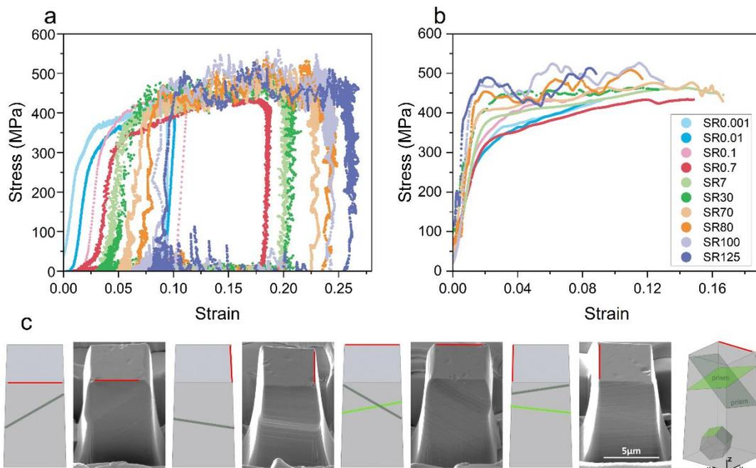
Figure 8 (a) The coupled engineering stress-strain curves for micropillar compression tests in P2 at both NSR and HSR. [Each test has shifted slightly along the X axis to aid visualisation.] (b) Smoothed stress-strain curves of the coupled P2 results; (c) SE micrographs and 3D models showing the relationship between pillars and slip planes for the four sides of the deformed pillar P2 at strain rate 70. [The red line annotation indicates the same pillar vertex for each micrograph.]
