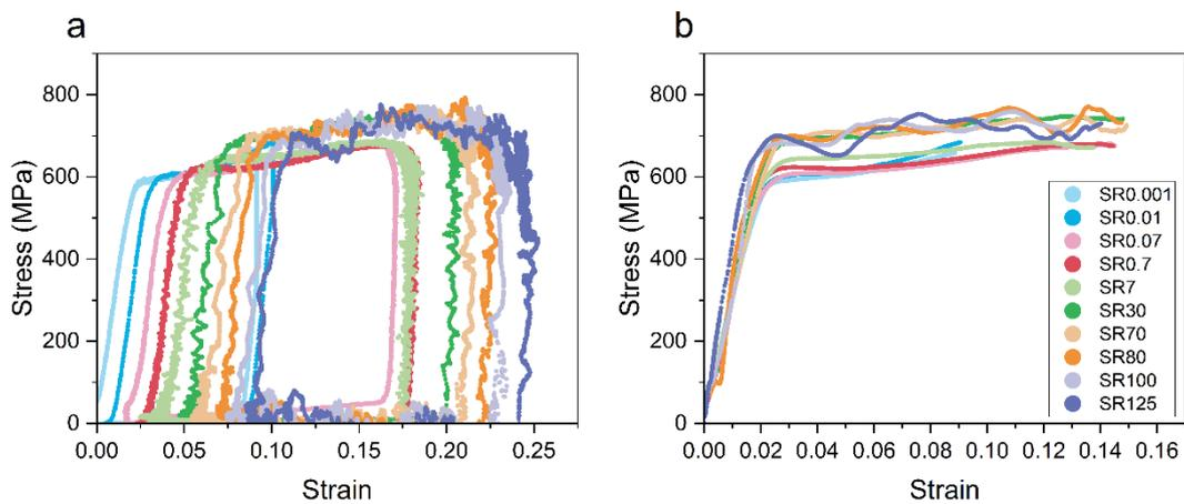
Figure 4 (a) The coupled engineering stress-strain curves for micropillar compression tests in B1 at both NSR and HSR. [Each test has shifted slightly along the X axis to aid visualisation.] (b) Smoothed stress-strain curves of the coupled B1 results.
