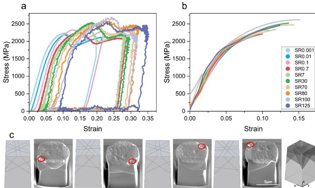
Figure 10 (a) The coupled engineering stress-strain curves for micropillar compression tests in PY at both NSR and HSR. [Each test has shifted slightly along the X axis to aid visualisation.] (b) Smoothed stress-strain curves of the coupled PY results; (c) SE micrographs and 3D models showing the relationship between pillars and slip planes for the four sides of the deformed pillar PY at strain rate 125. [The red line annotation indicates the same pillar vertex for each micrograph.]
