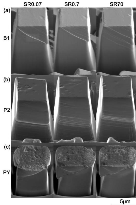
Figure 13 SE micrographs showing post-deformation micropillars in different grains B1, P2 and PY, compressed with different strain rates. [The SE micrographs of the other 3 sides of the pillar can be found in Supplementary.]
