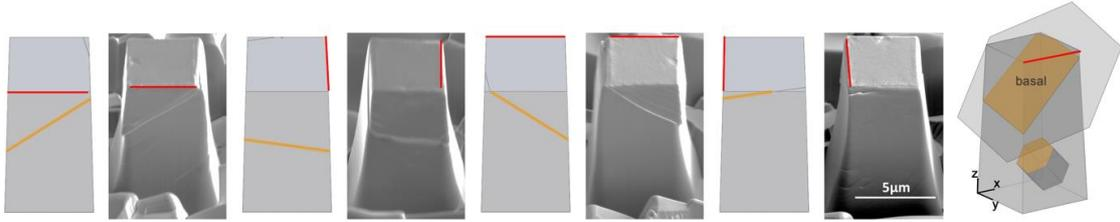
Figure 5 SE micrographs and 3D models showing the relationship between pillars and slip planes for the four sides of the deformed pillar B1 at a strain rate of 0.7. [The red line annotation indicates the same pillar vertex for each micrograph.]
