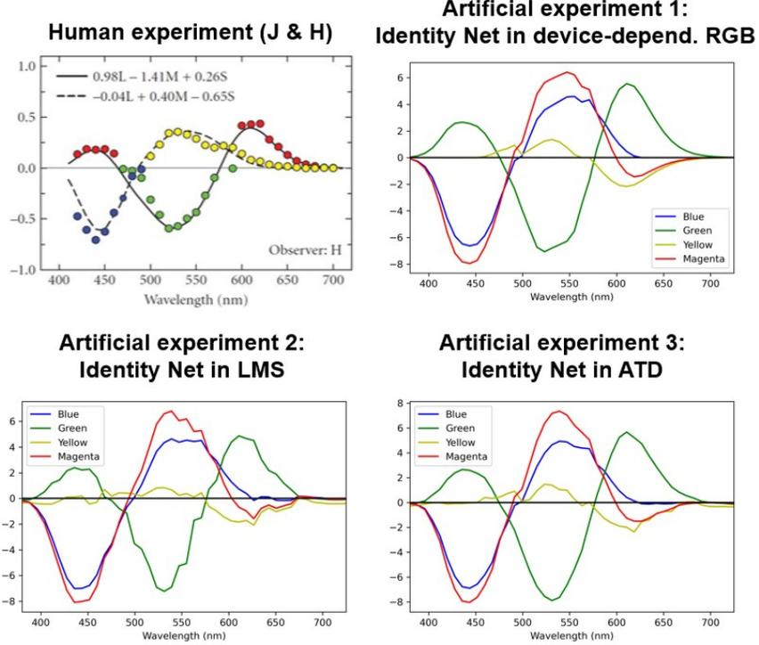
Figure 6: Optimal weights,  $w_i^*(\lambda)$ , of the classical cancellation lights for the trivial identity network operating in different photoreceptor color spaces. Here we show the magenta curve (built from the blue curve and the red curve) that can be directly subtracted from the green curve to obtain  $V_{RG}$
