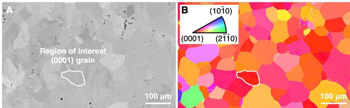
**Figure 1.** (a) Backscatter electron image where the region of interest is marked. (b) Inverse pole figure from EBSD mapping. A grain with (0001) surface was chosen based on the corresponding inverse pole figure from EBSD mapping.
