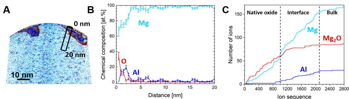
**Figure 8.** (a) 4 nm slice of Mg-2Al-0.1Ca evaporated in voltage mode with indication of the 4x4x20 nm cylindrical profile. (b) Concentration profile of cylindrical region indicated in (a) for magnesium, aluminum and oxygen. (c) Cumulative plot of number of ions vs. ion sequence for Mg, Mg<sub>2</sub>O and Al ions.
