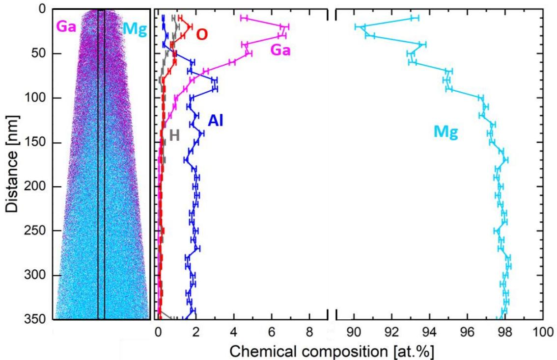
**Figure 2.** Reconstructed APT specimen of Mg-2Al-0.1Ca during the gallium cleaning step with an indication of specimen length and corresponding chemical composition along the drawn-in 350x10x10 nm cylinder.
