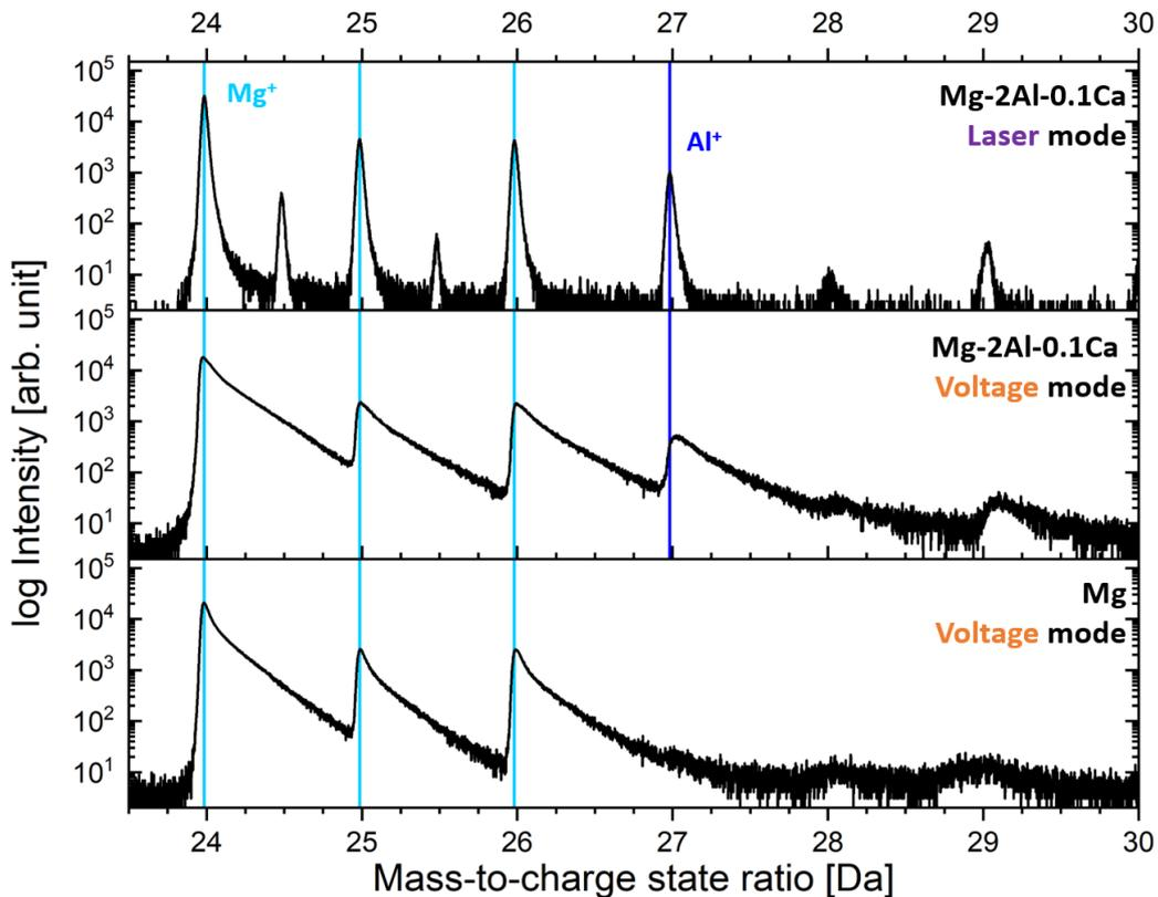
**Figure 6.** Detailed mass spectrum data in the range of 23 to 30 Da of Mg-2Al-0.1Ca oxidized in ambient air for 12 h measured in laser and voltage mode and magnesium reference sample oxidized in air for 11 days measured in voltage mode. Cyan and blue lines represent the abundance of Mg<sup>+</sup> and Al<sup>+</sup> isotopes, respectively.
