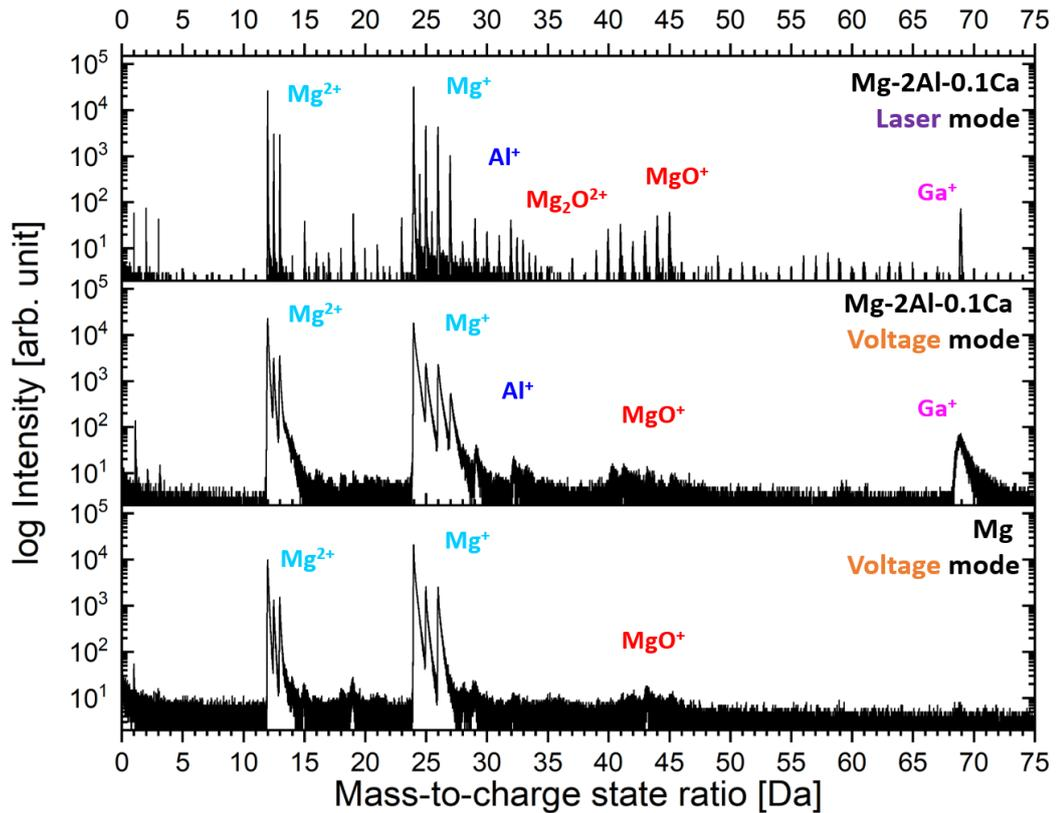
**Figure 5.** Mass spectra for Mg-2Al-0.1Ca oxidized in ambient air for 12 h measured in laser and voltage mode and the magnesium reference sample oxidized in air for 11 days measured in voltage mode. Peak positions for Mg<sup>2+</sup> and Mg<sup>+</sup> and their isotopes at 12 and 24 Da, respectively, Al<sup>+</sup> at 27 Da, Mg<sub>2</sub>O<sub>2</sub><sup>2+</sup> and MgO<sup>+</sup> with their isotopes at 32 and 40 Da, respectively, as well as Ga<sup>+</sup> at 69 Da are indicated.
