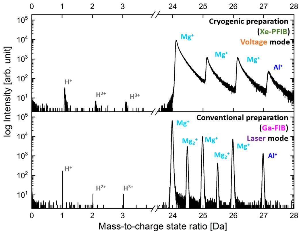
**Figure 3.** Mass spectra of Mg-2Al-0.1Ca after lift-out and sharpening with xenon PFIB and gallium FIB in a range from 0 to 4 Da with indication of hydrogen ions and from 23 to 28 Da with indication of  $\text{Mg}^+$  and  $\text{Mg}_2^{2+}$  and their isotopes, as well as  $\text{Al}^+$ . For both datasets 3.5 million ions were collected.
