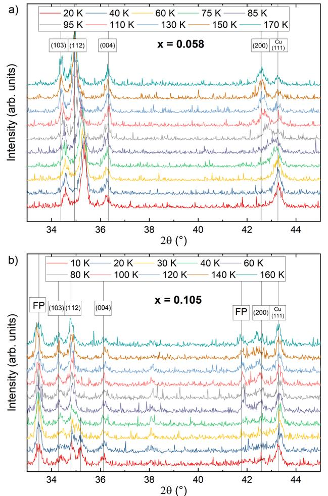
FIG. 6. Temperature dependent PXRD data for a)  $x = 0.058$  (valence fluctuating) and b)  $x = 0.104$  (antiferromagnetic). Reflexes are indexed, FP indicates reflexes originating from a foreign phase and Cu marks the reflex from the sample holder.
