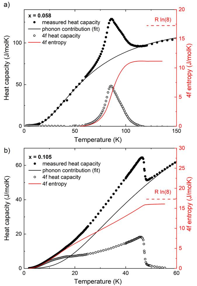
FIG. 5. Measured heat capacity (solid symbols), phonon background derived from a Debye-fit (black line), derived 4f-based heat capacity (open symbols) and resulting 4f entropy contribution (red line, right axis) in samples with a)  $x = 0.058$  (valence fluctuating) and b)  $x = 0.105$  (antiferromagnetic).
