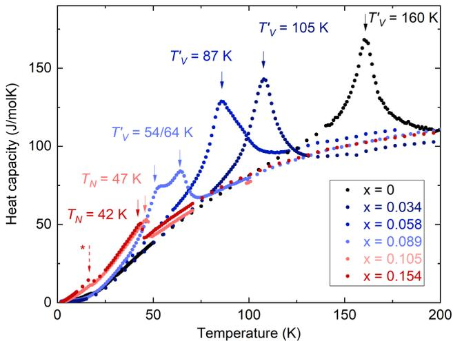
FIG. 4. Heat capacity for single crystalline  $\text{EuPd}_2(\text{Si}_{1-x}\text{Ge}_x)_2$  for varying  $x$  as specified in the figure. Blue arrows mark the position of the characteristic temperature of a valence crossover, whereas red arrows mark the Néel temperature of the antiferromagnetic transition. The dashed arrow with a star denotes an anomaly, assigned to the impurity phase, also seen in the susceptibility data.
