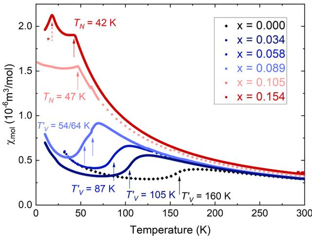
FIG. 2. Magnetic susceptibility data for different substituted samples at  $B = 0.1$  T and  $B \parallel c$ . Black and blue arrows mark the valence crossover at  $T'_V$ , while red arrows indicate the antiferromagnetic transition at  $T_N$ . The dashed arrow with a star denotes a magnetic transition from a foreign phase in the sample with  $x = 0.154$ .
