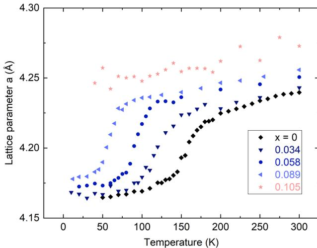
FIG. 7. Temperature dependence of the lattice parameter  $a$  for different Ge-substitution levels in  $\text{EuPd}_2(\text{Si}_{1-x}\text{Ge}_x)_2$ . The shown data is obtained by refinement of the temperature dependent PXRD data.
