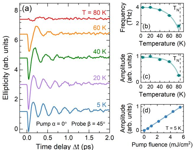
FIG. 2. (a) Transient probe ellipticity at different temperatures below  $T_N = 83$  K. Pump and probe pulses are linearly polarized at angles  $\alpha = 0^\circ$  and  $\beta = 45^\circ$ , respectively. Temperature dependences of the (b) frequency and (c) amplitude of the oscillations seen in (a). (d) Dependence of the amplitude of the oscillations on the pump pulse fluence at  $T = 5$  K. The solid lines in (b-d) are guides for the eye.
