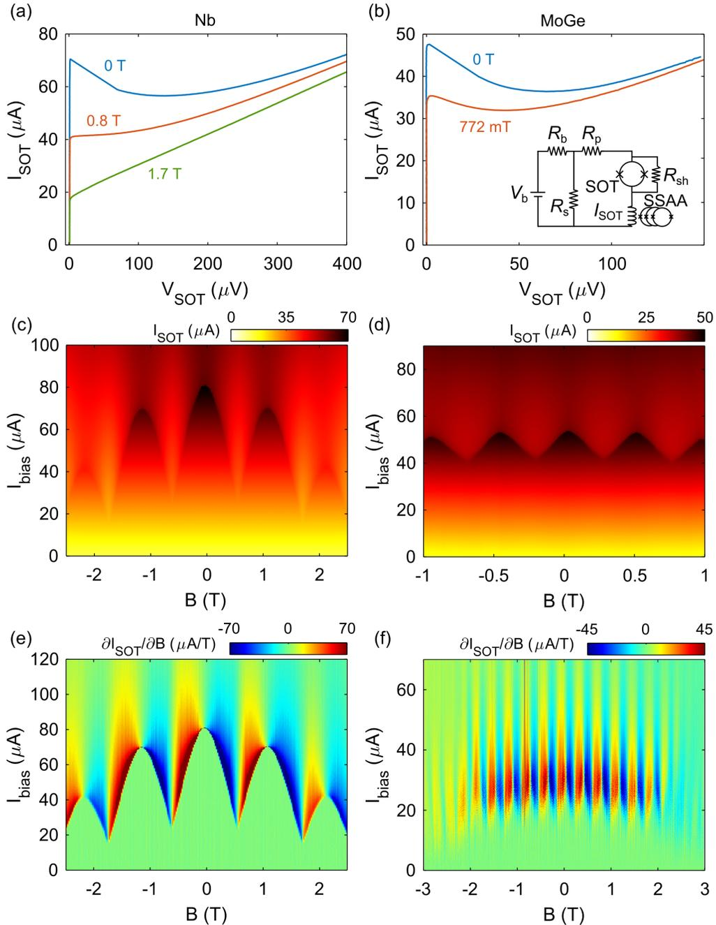
Figure 2: Current-voltage characteristics at 4.2 K. Current through the SQUID-on-tip  $I_{\text{SOT}}$  as a function of the voltage across it  $V_{\text{SOT}}$  at different magnetic fields applied along the probe axis for (a) Nb ( $R_p = 0.7 \Omega$ ,  $R_{\text{sh}} = 5 \Omega$ ) and (b) MoGe ( $R_p = 0.5 \Omega$ ,  $R_{\text{sh}} = 7 \Omega$ ) devices. The inset shows a simplified diagram of the electronic circuit used.
