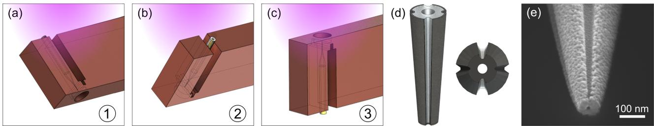
Figure 1: Illustration of the SQUID-on-tip holder for magnetron sputtering deposition. The holder is rotated at deposition angles of (a)  $+120^\circ$ , (b)  $-120^\circ$ , and (c)  $0^\circ$ , with respect to the direction of the sputtering source. The plasma is schematically shown in purple. (d) Schematic drawing of a pulled four-groove capillary after film deposition with views from the side and bottom. (e) SEM micrograph of a Nb SQUID-on-tip with geometrical diameter of 55 nm.
