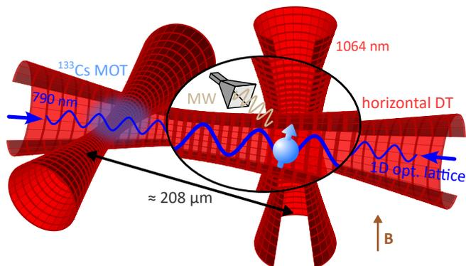
FIG. 1. **Sketch of the experimental setup.** Three running dipole trapping beams at a wavelength of 1064 nm (red) build two independent crossed optical dipole traps sharing one trapping beam along the horizontal direction. The one-dimensional optical lattice (dark blue) is a standing-wave dipole trap formed by a pair of laser beams at a wavelength of 790 nm superimposed with the shared horizontal dipole trap. Microwave (MW) radiation couples the Cs clock states.
