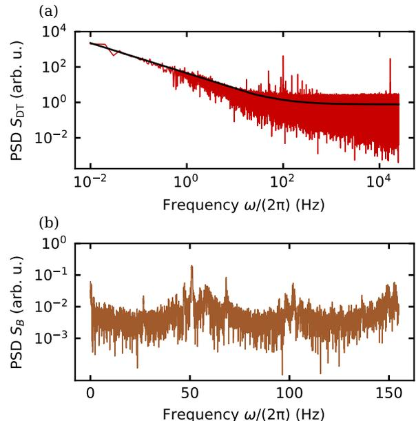
FIG. 7. **Environmental noise characterization** (a) PSD of the output signal from a fast photodiode when laser light of the horizontal dipole trap is shown onto it. The solid line shows a fit according to Eq. (29), yielding an exponent  $\tilde{\alpha} = 0.8904(2)$ . (b) PSD of the current through the magnetic field coils.
