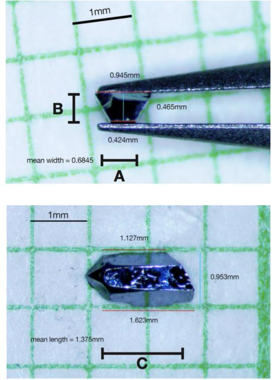
FIG. 8. Most of the magnetic measurements were done on the  $\text{LaCrGe}_3$  crystal pictured. One side was lightly polished flat and parallel to the opposite face. We determined the size from pictures of the sample on mm grid paper. From these measurements we were able to estimate the demagnetization factors  $N_a$ ,  $N_b$  and  $N_c$ .
