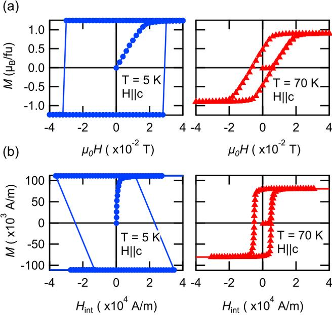
FIG. 9. (a)  $M \nu H$  curves and (b) the demagnetization corrected  $M \nu H_{\text{int}}$  curves. By taking into account the demagnetization field resulting from the finite size of our magnetized sample, we can plot magnetization against the internal field  $H_{\text{int}}$ .
