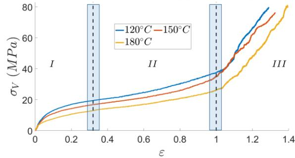
Figure S6 True strain-true stress curves ( $\sigma_v(\varepsilon)$ ).
