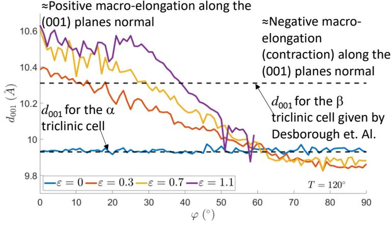
Figure 13  $d_{001}$  versus the azimuthal angle along the (001) reflection ring at different strains. At  $\varepsilon = 1.1$ , the ring intensity becomes very weak for  $\varphi > 60^\circ$  and  $d_{001}$  cannot be measured.
