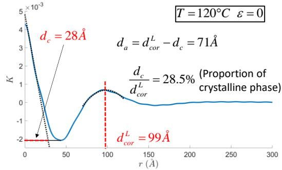
Figure S4 Illustration of the procedure to obtain  $d_c$  (thickness of lamellae),  $d_a$  (thickness of amorphous layers) and the proportion of crystalline phase through the characteristics of  $K(r)$  ([Strobl (1980)]) for our PBT at 120°C and  $\varepsilon = 0$ .
