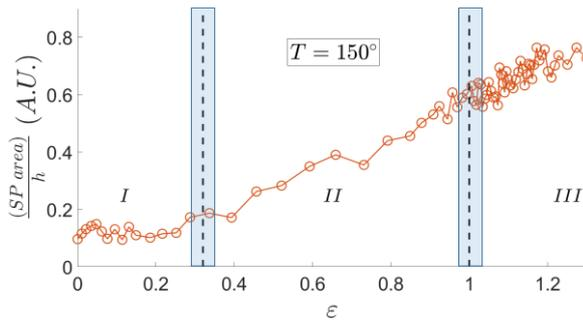
Figure S17 Area of SP (new peak associated with the smectic phase) normalized by the specimen thickness ( $h$ ) versus  $\varepsilon$  ( $150^{\circ}\text{C}$ ).
