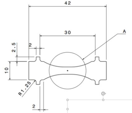
Figure S2 Specimen dimensions.
