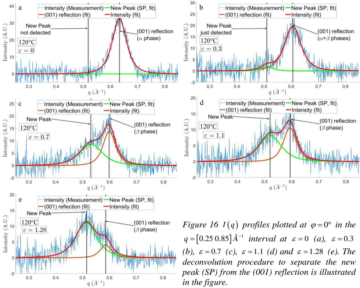
Figure 16  $I(q)$  profiles plotted at  $\varphi = 0^\circ$  in the  $q = [0.25 \ 0.85] \text{\AA}^{-1}$  interval at  $\varepsilon = 0$  (a),  $\varepsilon = 0.3$  (b),  $\varepsilon = 0.7$  (c),  $\varepsilon = 1.1$  (d) and  $\varepsilon = 1.28$  (e). The deconvolution procedure to separate the new peak (SP) from the (001) reflection is illustrated in the figure.
