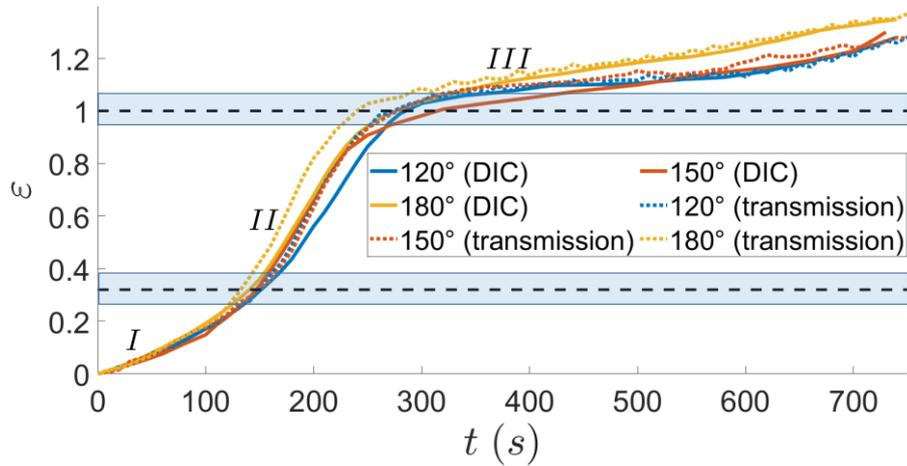
Figure S3 Evolution of true strain ( $\epsilon(t)$ ) measured in the specimen central cross-section. Comparison between the DIC measurements and those obtained independently during the in situ X Ray scattering experiments from the transmission signal. Using the beer Lambert-Law and the assumption of isochoric deformation process, it is easy to check that:
