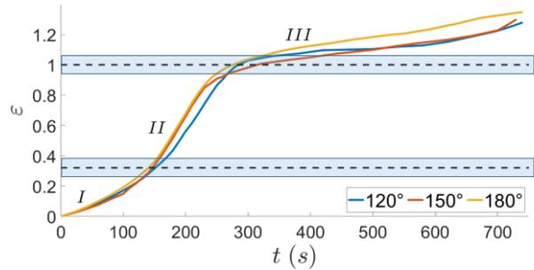
Figure 2 Evolution of the true longitudinal strain  $\varepsilon(t)$  measured in the specimen central cross-section
