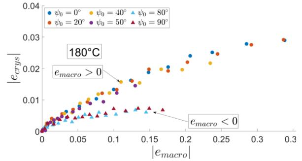
Figure S14 Local elongations versus macro-elongations. Results provided in absolute values ( $T=180^{\circ}\text{C}$ ).
