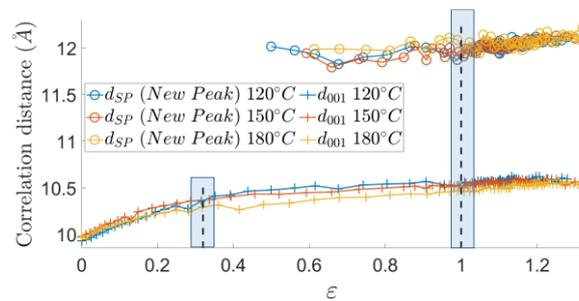
Figure S16 Evolution of the correlation distance for the (001) reflection and the new peak corresponding to the smectic phase (obtained from the  $I(q)$  profiles averaged in the  $\varphi = [0\ 5]^{\circ}$  interval).
