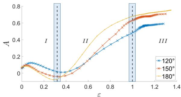
Figure 7 Orientation parameters extracted from the SAXS patterns.
