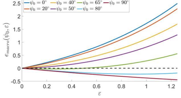
Figure A2 Evolution of the macro-elongation  $e_{macro}(\psi_0, \varepsilon) = \frac{\ell^{\psi}(\varepsilon) - \ell^{\psi_0}(0)}{\ell^{\psi_0}(0)}$  for a length element  $\ell^{\psi_0}$  initially making an angle  $\psi_0$  with respect to the drawing axis
