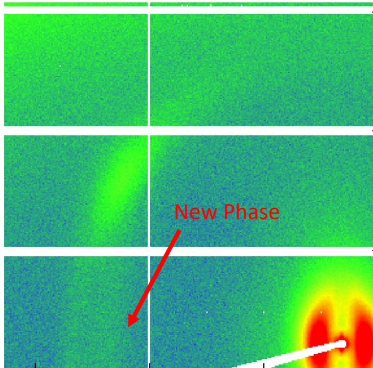
Figure S15 Pattern measured at  $120^{\circ}\text{C}$  and  $\varepsilon = 1.1$ . Compared to Figure 13, the noise threshold was lowered to make the new peak associated with the new phase easier to observe.
