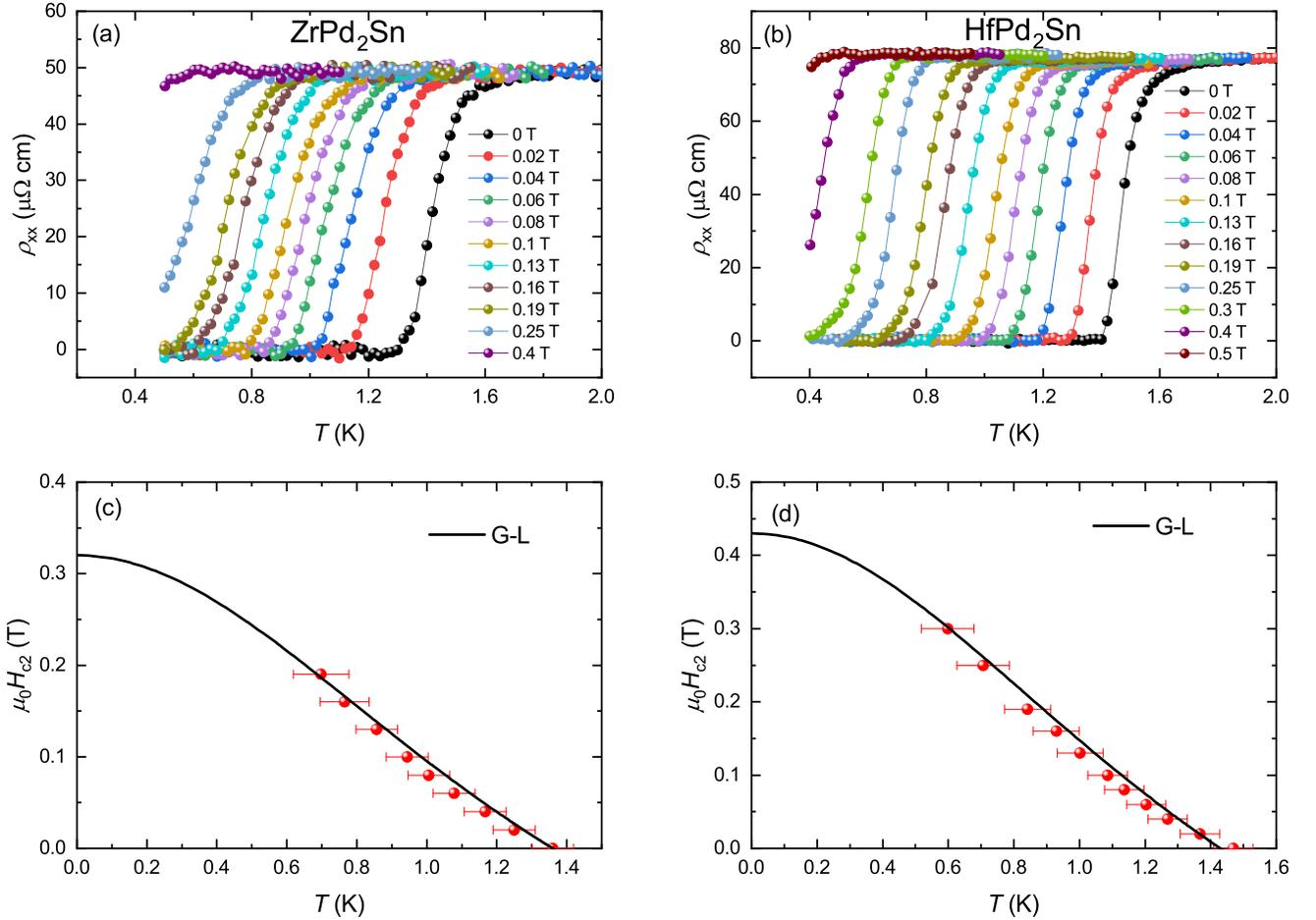
FIG. 7. (Color online) (a), (b): Temperature dependence of the electrical resistivity of  $\text{ZrPd}_2\text{Sn}$  and  $\text{HfPd}_2\text{Sn}$ , measured under various applied magnetic fields in the vicinity of  $T_c$ . The upper critical fields  $\mu_0 H_{c2}(T)$  are shown in (c) and (d),  $T_c$  was determined from the midpoint of the resistivity drop at the transition. The solid lines correspond to fitting using the Ginzburg-Landau (G-L) model.
