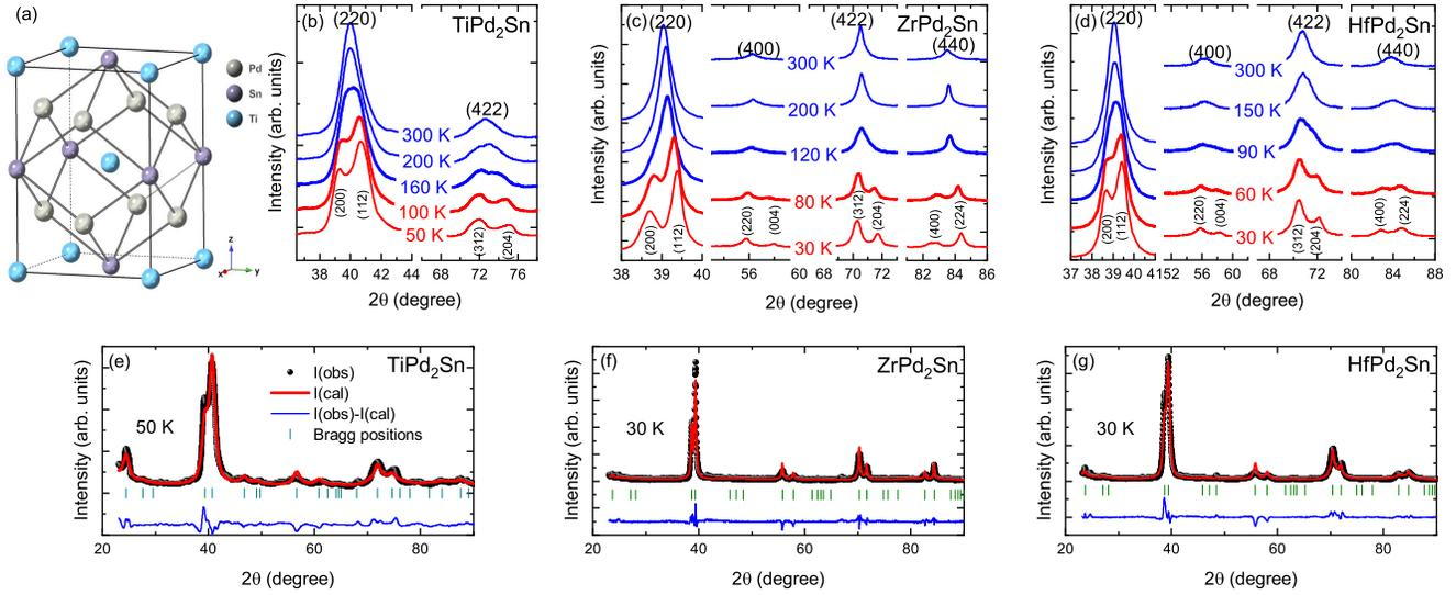
FIG. 4. (Color online) (a) Low temperature tetragonal crystal structure of  $\text{TiPd}_2\text{Sn}$ . (b), (c) and (d): powder x-ray diffraction patterns of  $\text{XPd}_2\text{Sn}$  ( $X = \text{Ti}, \text{Zr}, \text{Hf}$ ) measured at various temperatures, focusing on a few major diffraction peaks. The corresponding powder x-ray diffraction patterns together with the calculated results from Rietveld refinements at the lowest measured temperatures ( $T < T_s$ ) are shown in (e), (f) and (g).
