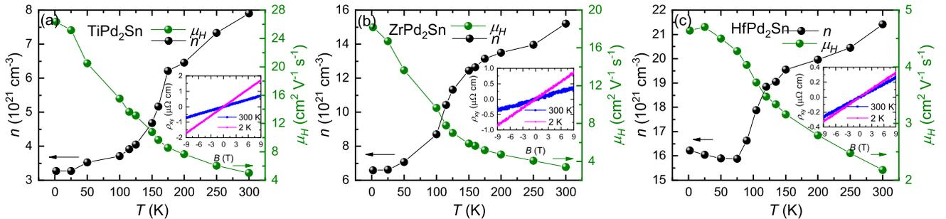
FIG. 3. (Color online) The temperature dependence of the carrier density and mobility of the Hall resistivity of (a)  $\text{TiPd}_2\text{Sn}$ , (b)  $\text{ZrPd}_2\text{Sn}$  and (c)  $\text{HfPd}_2\text{Sn}$ . The field-dependence of the Hall resistivity at two temperatures are shown in the insets.
