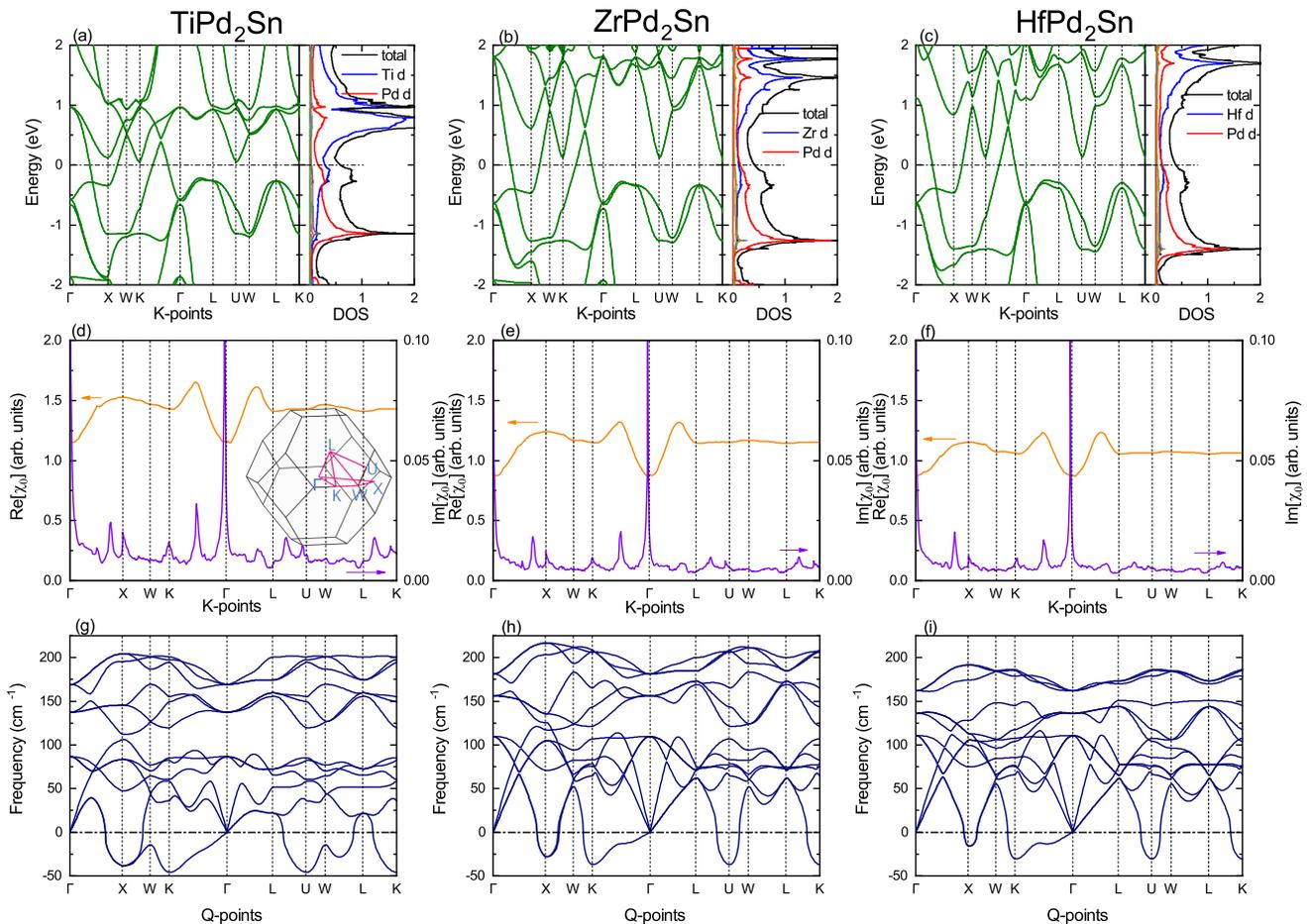
FIG. 8. (Color online) DFT calculations of  $XPd_2Sn$  ( $X = Ti, Zr, Pd$ ). (a), (b) and (c): electronic band structure and density of states, taking into account spin-orbit coupling (SOC). (d), (e) and (f): bare electron susceptibility  $\chi_0$ , where the orange (purple) solid lines denote real (imaginary) parts. Inset of (d): Brillouin zone and high symmetry points, and (g), (h) and (i): Phonon spectra of the three compounds.
