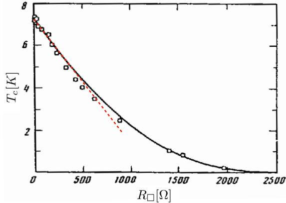
Figure 11: Suppression of superconductivity in amorphous  $\text{Mo}_{79}\text{Ge}_{21}$  [47]. The solid line is a theoretical fit obtained from the RG equation for  $\gamma_c$  in Ref. [28]. The red dashed line highlights the rapid initial decrease of the  $T_c$ - $R_{\square}$  curve.
