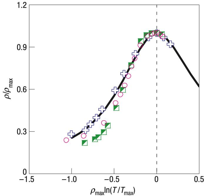
Figure 12: The RG-fitting of the resistivity in a Si-MOSFET device [72]. The data corresponding to densities  $n = (9.87, 9.58, 9.14) \times 10^{10} \text{cm}^{-2}$  presented in Fig. 13 are scaled according to the universal solution given by Eq. (39); no adjustable parameters have been used to fit the data. The solid line (in black) is the universal solution  $R(\eta)$  of the pair of the RG equations (38a and 38b) with  $n_v = 2$ .
