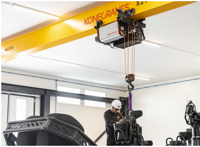
Fig. 1. The fiber rope crane used in this work. The photo is published with permission from Konecranes [8].
