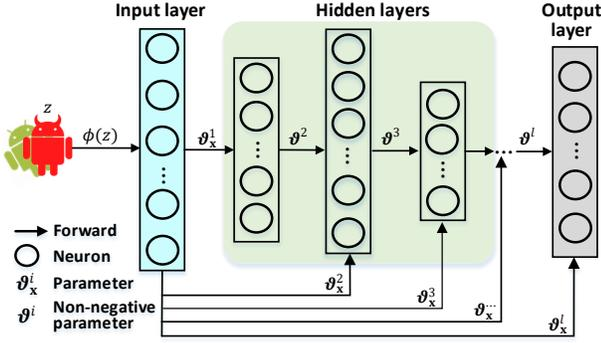
Fig. 4: Architecture of an input convex neural network.
