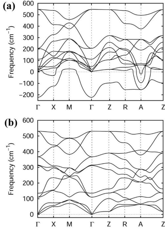
FIG. 3. Phonon spectrum of (a) the nonpolar and (b) the polar BiNiO<sub>2</sub> along the  $\Gamma(0, 0, 0)$ -X(0, 0.5, 0)-M(0.5, 0.5, 0)- $\Gamma$ -Z(0, 0, 0.5)-R(0, 0.5, 0.5)-A(0.5, 0.5, 0.5)-Z directions. The imaginary frequencies are indicated as negative values.
