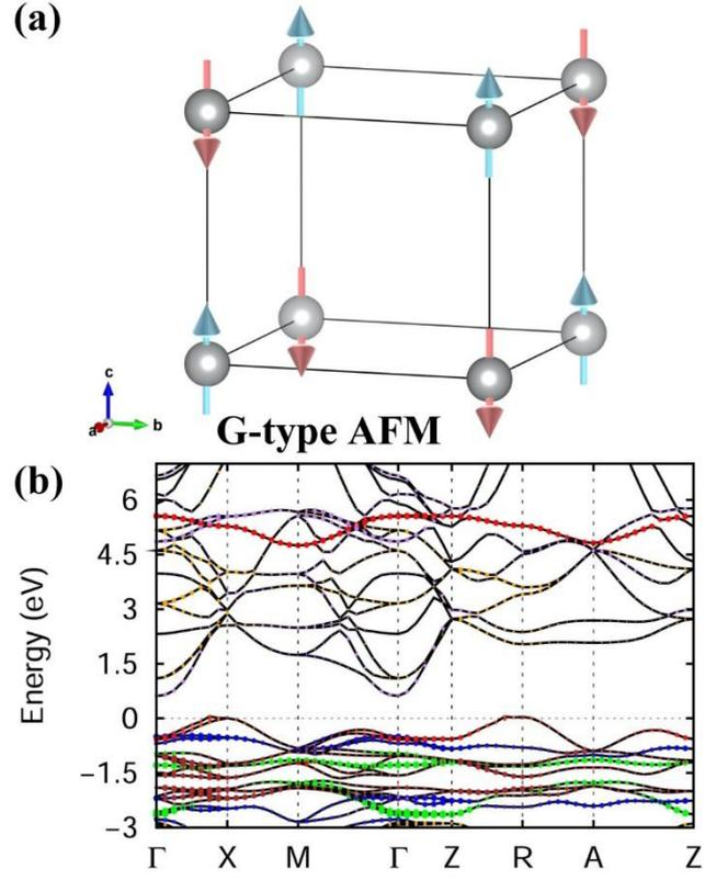
FIG. 9. (a) The G-type of antiferromagnetic (AFM) order. (b) HSE06 band structures of G-type AFM states for a  $\sqrt{2} \times \sqrt{2} \times 2$  supercell in the polar BiNiO<sub>2</sub>. The color has the same meanings as in Fig. 4.
