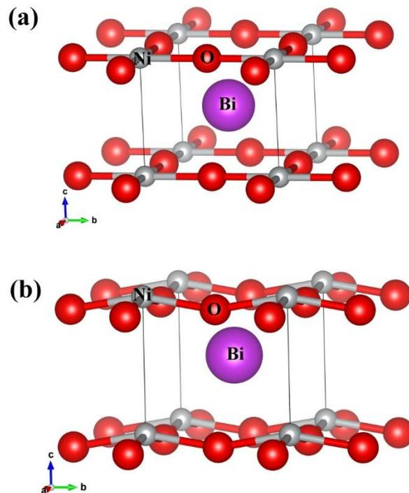
FIG. 2. The crystal structures of (a) the nonpolar BiNiO<sub>2</sub> with the  $P4/mmm$  symmetry (No. 123) and (b) the polar BiNiO<sub>2</sub> with the  $P4mm$  symmetry (No. 99).
