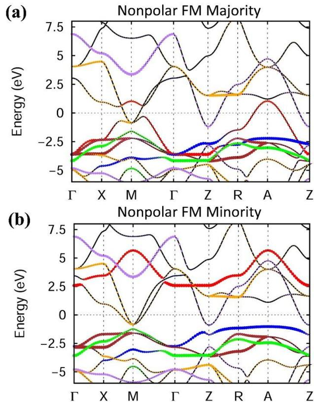
FIG. 7. HSE06 band structures of the ferromagnetic state of the spin (a) majority (b) minority
