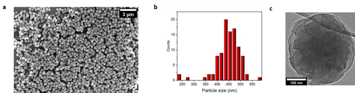
**Figure S2.** TABP-PDA COF particle morphology and structure. **a:** SEM image illustrating uniform size distribution of the washed COF microparticles. **b:** Particle size distribution showing high uniformity. **c:** TEM image showing a single COF nanoparticle consisting of crystalline domains with a lateral size of approx. 50 nm.
