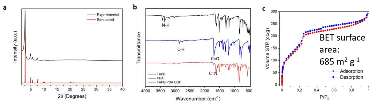
**Figure S1.** TABP-PDA COF structural analysis. **a:** Powder XRD after washing. **b:** FT-IR of the precursors and the COF. **c:** BET surface area measurement for overall surface area analysis.
