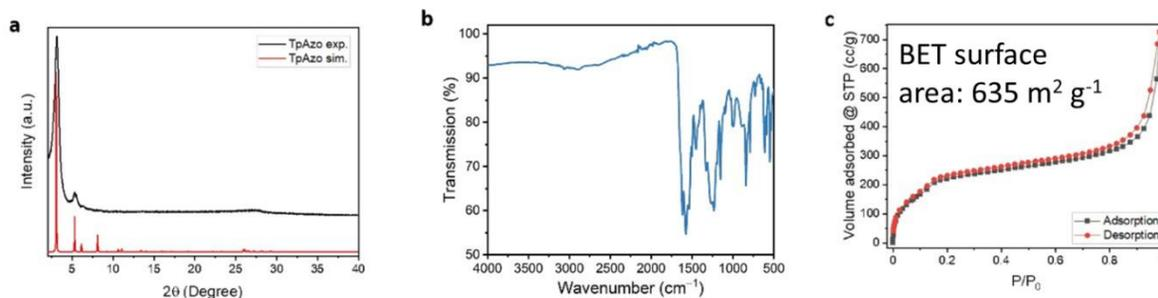
**Figure S3:** TpAzo-COF structural analysis. **a:** Powder XRD after washing. **b:** FTIR of the COF. **c:** BET surface area measurement for overall surface area analysis.
