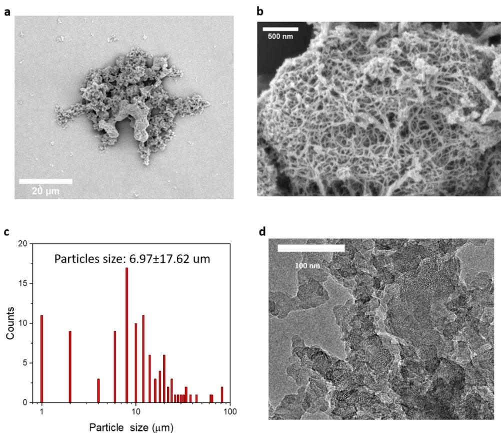
**Figure S4.** TpAzo-COF particle morphology and structure. **a:** SEM image illustrating the agglomerated structure of TpAzo-COF microparticles. **b:** SEM image (zoomed in) showing sponge-like inner structure with macropores. **c:** Particle size distribution showing non-uniformity of the particle agglomerates. The particle size is centered around 7  $\mu\text{m}$ . **d:** TEM image showing the interconnection of crystalline COF nanosheets with a domain size of approximately 50 nm or less.
