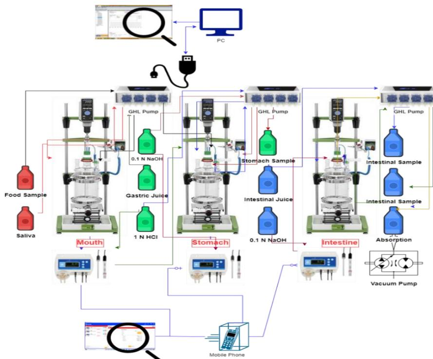
Figure 3.4. Design of Automatic in-vitro digestive system for evaluating bio-accessibility and release kinetics of lycopene-PLGA/PLA nanoparticles.
