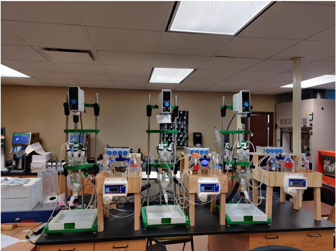
Figure 4.39. The AK-AutoGIT automatic programmable simulator of the human digestive system.
