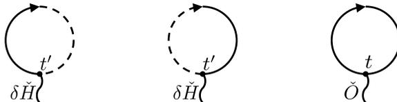
Figure C.11: Disconnected loop diagrams featuring in the linear response formulas. The left two diagrams are the retarded and advanced loops, the sums of which cancel. The rightmost diagram is the Keldysh loop, which generically always appears as a prefactor in front of cancelling terms.
