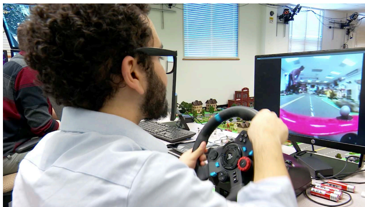
Figure 5: A driver emulation station interfaced directly with the robotics vehicles.
