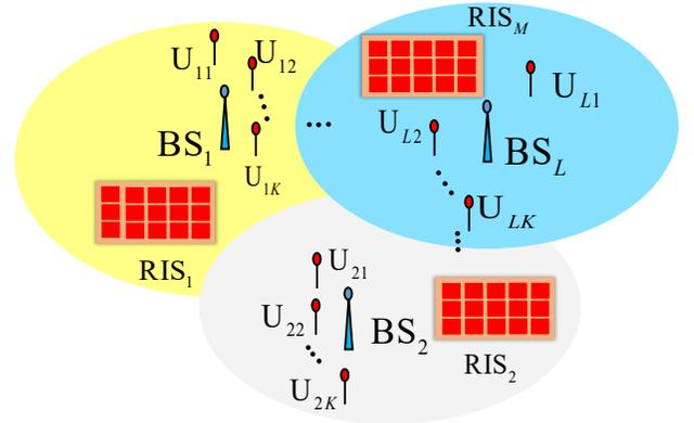
**Fig. 1:** A multicell broadcast channel with RIS.
