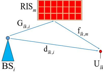
Fig. 2: Channel model in a typical RIS-assisted system.
