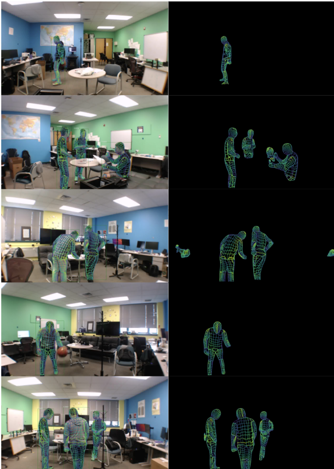
Figure 9: Qualitative comparison using synchronized images and WiFi signals. (Left Column) image-based DensePose (Right Column) our WiFi-based DensePose.
