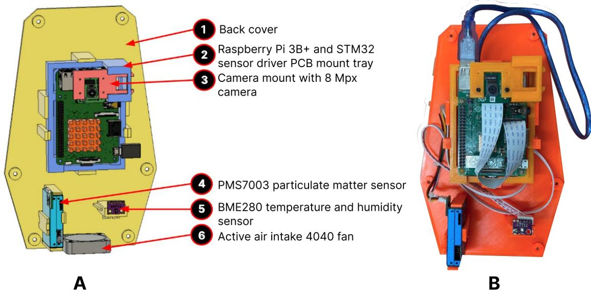
Figure 1: A single integrated air sensing hardware system. A - Computer-aided design, B - Real wired design.
