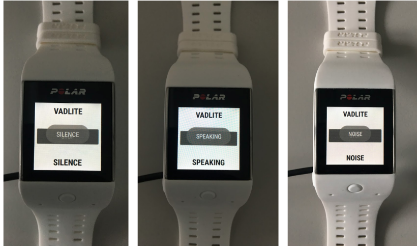
Fig. 10. Real-time testing of VADLite showing detection states of silence (left), speech (middle) and noise (right)
