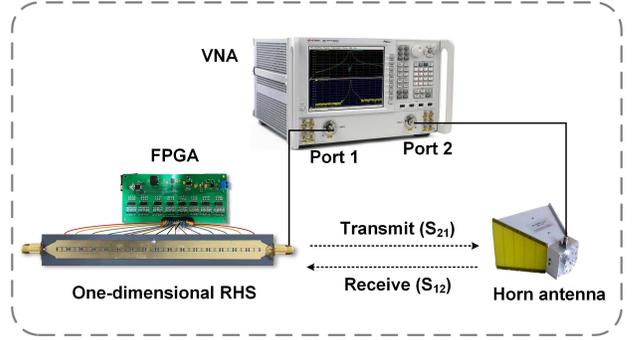
Fig. 4. Beam pattern measurement of the RHS.
