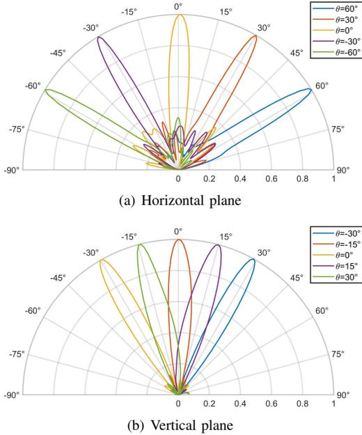
Fig. 3. Normalized far-field beam patterns of the RHS in the horizontal plane and the vertical plane.
