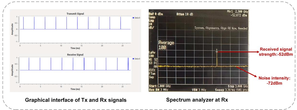
Fig. 7. Experimental results of RHS-aided point-to-point communications.
