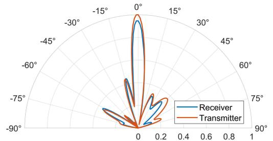
Fig. 6. Normalized far-field beam pattern of the RHS.
