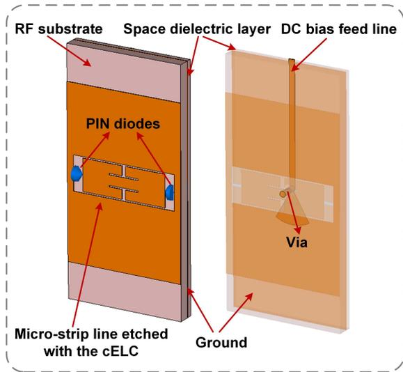
Fig. 2. Hardware design of the RHS element.
