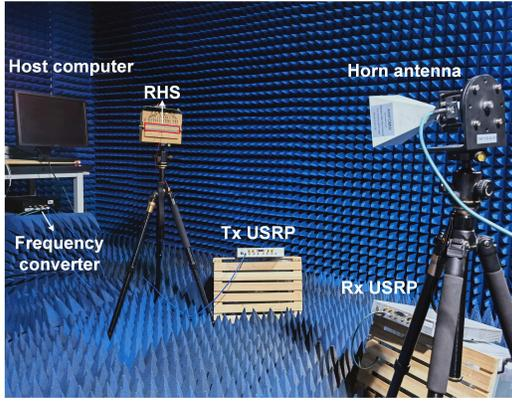
Fig. 5. RHS-aided point-to-point communication platform.
