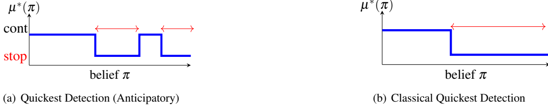
Figure 8: (a) The remarkable multi-threshold structure of quickest detection policy \mu^* as a function of belief (posterior) \pi in quickest detection with anticipatory agents. The stopping set is non-convex (disconnected) as shown in red. (b) The optimal policy in classical quickest detection is a single threshold with convex stopping set.
