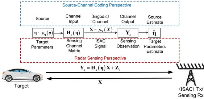
Fig. 2. Wireless sensing as non-cooperative joint source-channel coding.
