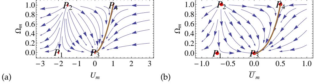
**Figure 10.** Phase plane for the system (6.11) showing both the stability of the background equations as well as the stability of the perturbations for the  $\Lambda$ CDM model. (a) in the original fractional energy density  $\Omega_m$  vs the phase of matter perturbations  $U_m$ . (b) Using the compact variables  $\Omega_m$  vs  $\frac{2}{\pi} \arctan(U_m)$ .
