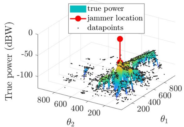
**Fig. 3.** Power measurements under ray tracing model propagation.
