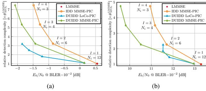
Fig. 6. Computational complexity vs. performance (measured in minimal SNR required to achieve BLER = 1%) trade-off for a fixed number  $N_{MP} = 12$  of total MP decoding iterations. The subfigures consider a MU-MIMO-OFDM system (a) with  $B \times U = 8 \times 4$  i.i.d. Rayleigh fading channels and perfect CSI, and (b) with  $B \times U = 16 \times 4$  ray-tracing channels and estimated CSI.
