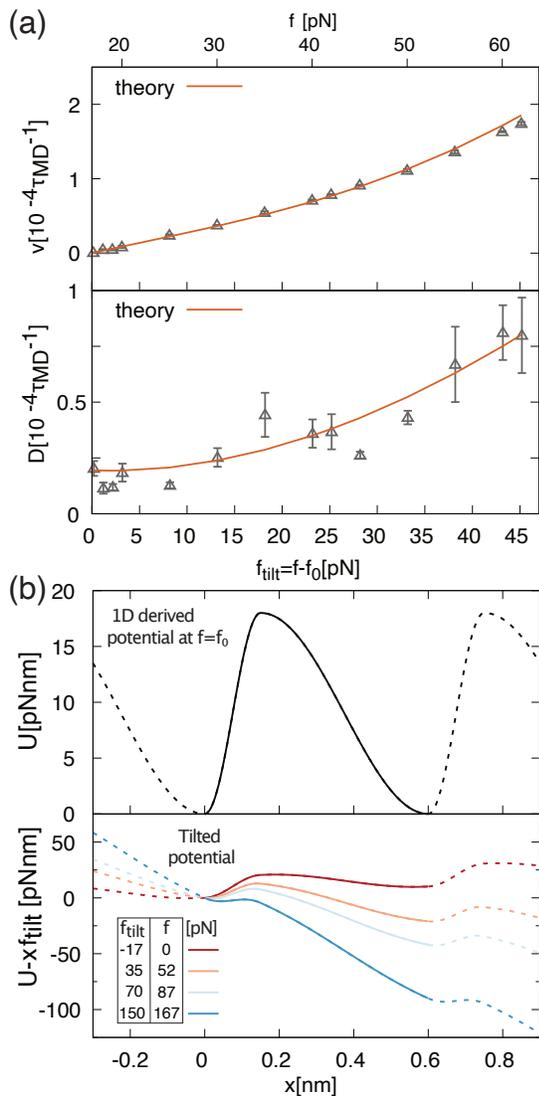
FIG. 3. Derivation of the unzipping potential from nonequilibrium data. The data points in panels (a) show the average velocity and diffusion coefficient of the nanopore unzipping process at different forces,  $f$ . The continuous theoretical curves are based on Eqs. 1 and correspond to the least-square fit of the data via an optimal parametrization of the washboard potential,  $U(x)$ , of Eqs. 2. The potential is shown in panel (b) with and without various tilting forces.
