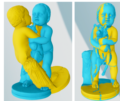
Fig. 14. "Enfant au Chien" ICP registration: without initialization (left) and with initialization (right).
