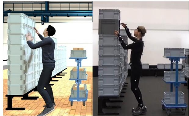
**Figure 2. Cyber-physical twin (left) of a real person-to-goods picking system (right).**
